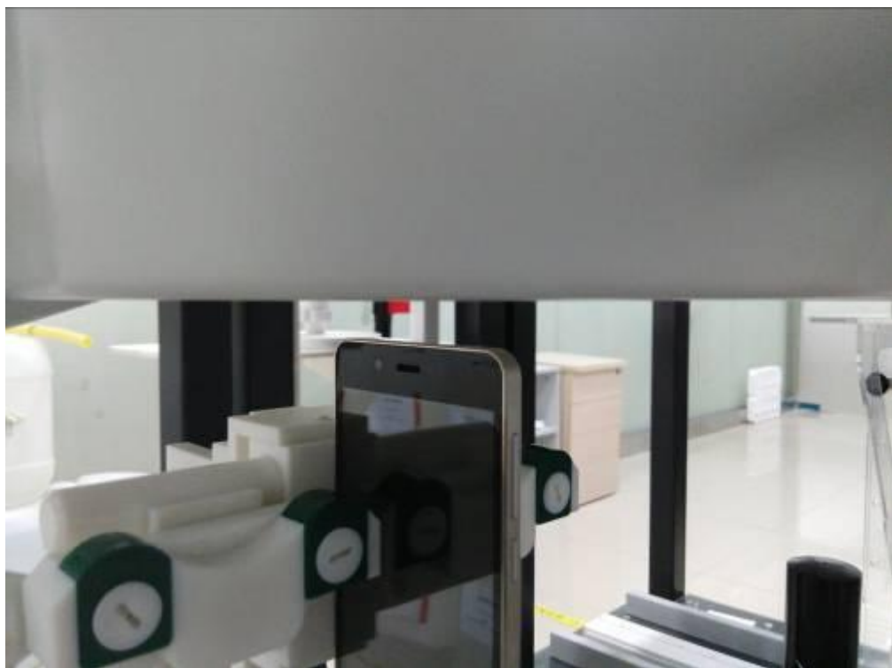
Body top side(separation distance is 10mm)
