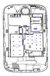
■ When you need to remove T-Flash card, please first turn off the phone, remove the battery, then remove the memory card.
