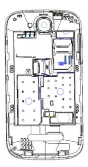
■ When you need to remove the SIM card, please first turn off the phone, remove the battery, then remove the SIM card.
