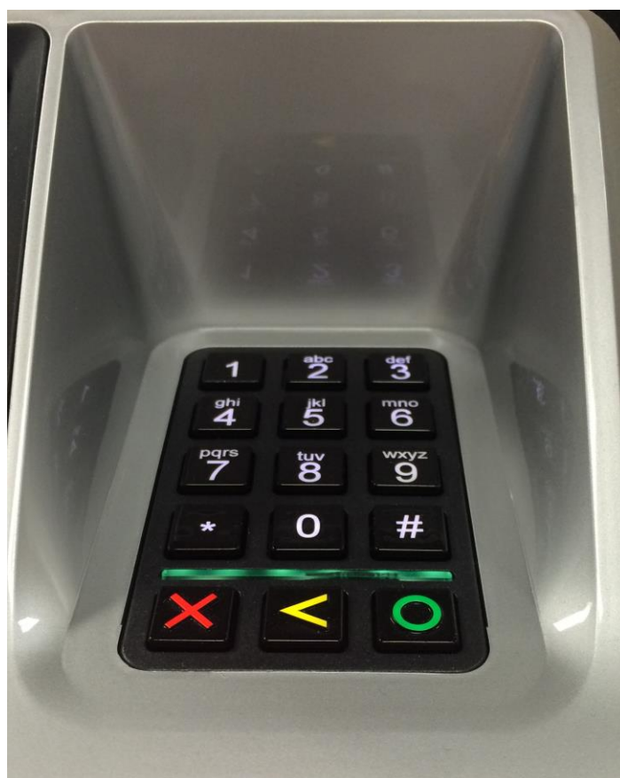
Key Pad and Privacy Shield
