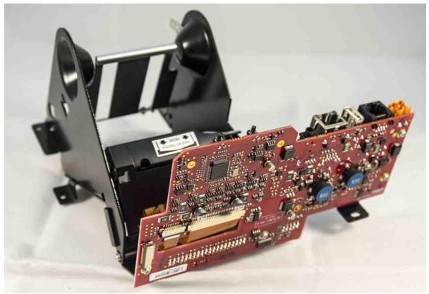
Figure 7 Power supply board and printer chute
