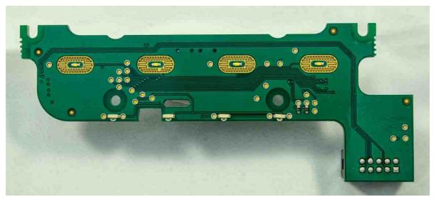
Figure 4 Contactless transceiver circuit board showing components from underneath
