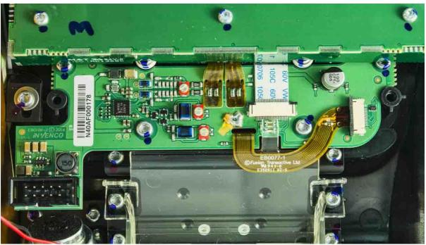
Figure 3 Contactless transceiver circuit board showing components from the top
