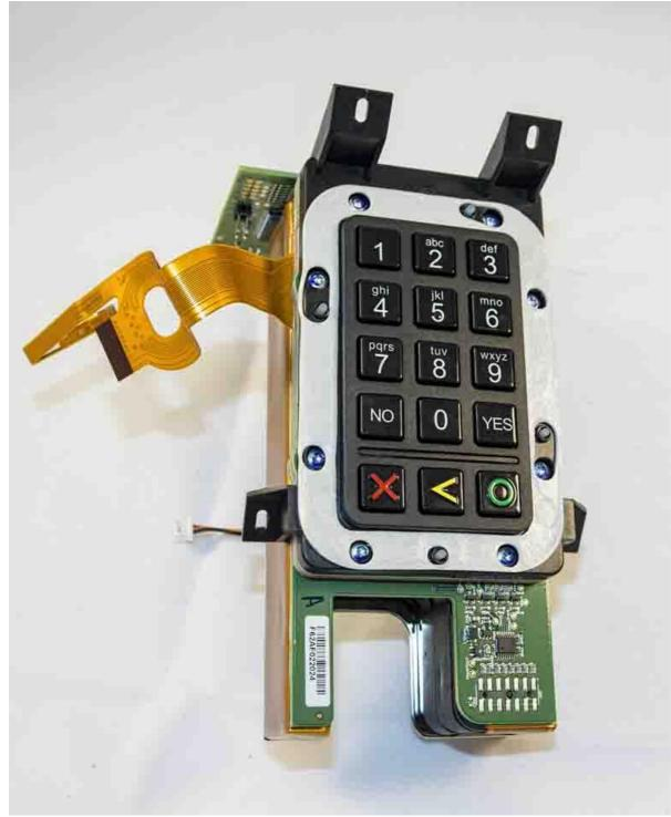
Figure 17 Unified Pin-pad and Card reader
