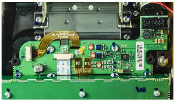
Figure 13 Contactless antenna board
