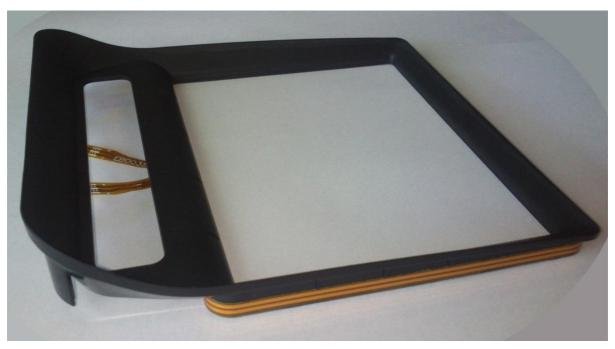
Figure 1 Bezel removed showing Contactless Circuit Antenna (Bezel up- Normal position)
