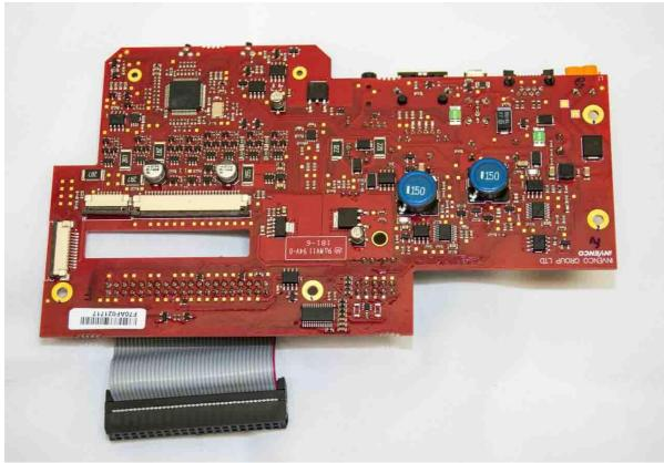
Figure 8 Power module topside
