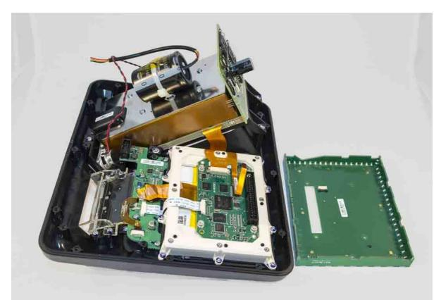
Figure 15 Security fence box removed exposing Secure Display Controller
