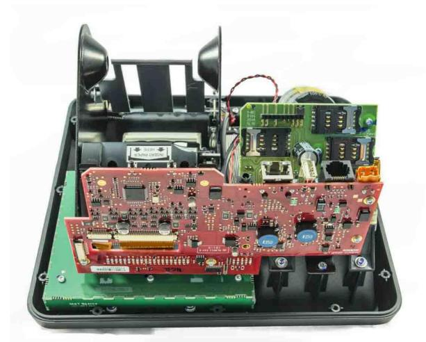
Figure 16 Completed electronic assembly without rear case
