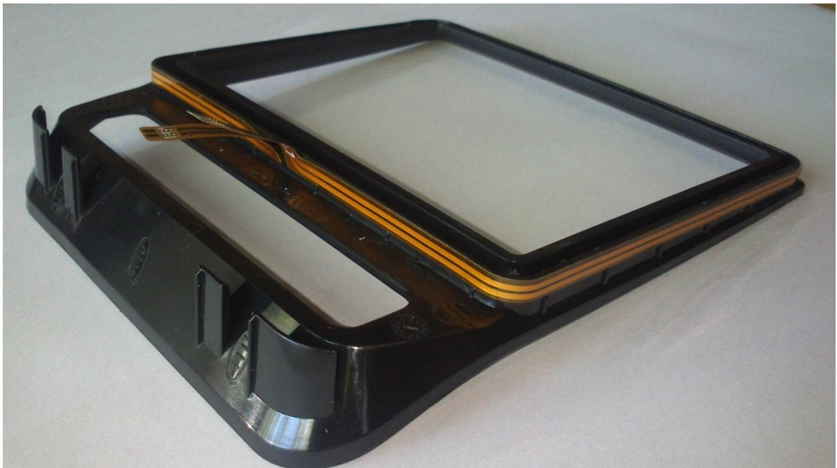
Bezel removed close up on rear side showing the contactless circuit antenna and antenna tail connection points that go to the circuit board.
