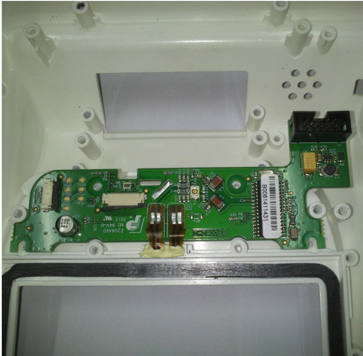
Contactless circuit board with the antenna tails connected
