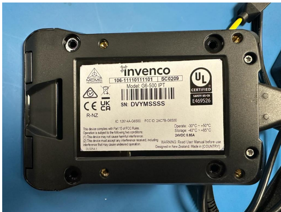
Figure 3, Model G6-500 IPT General label location - Rear side of the case
