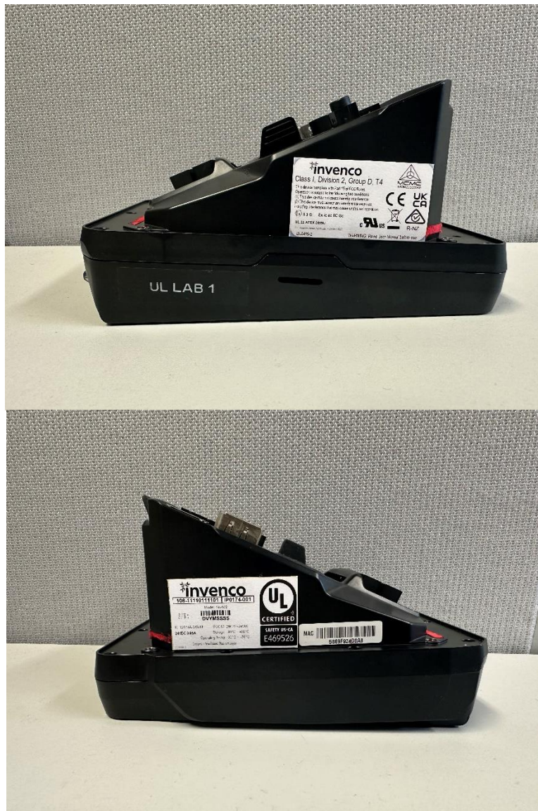
Figure 1, Model G6-500 General label location - both sides of the case
