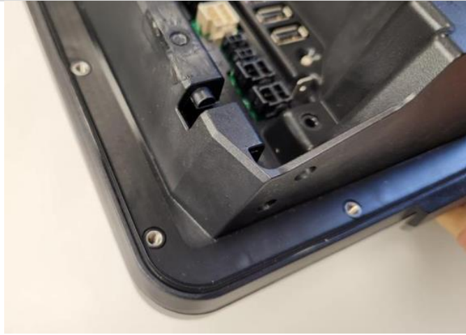
9.1: How to Attach the Gasket
