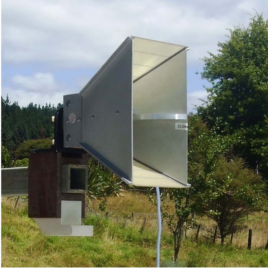
EMCO 3115 Horn Antenna (1 – 18 GHz)
