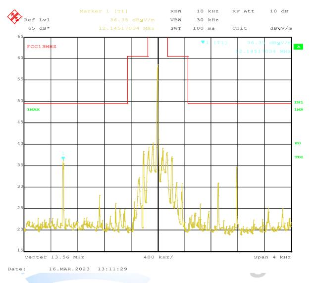
Measurement was made at the open area test site with high level ambient emissions detected and confirmed at 12.145 MHz and 14.742 MHz.
