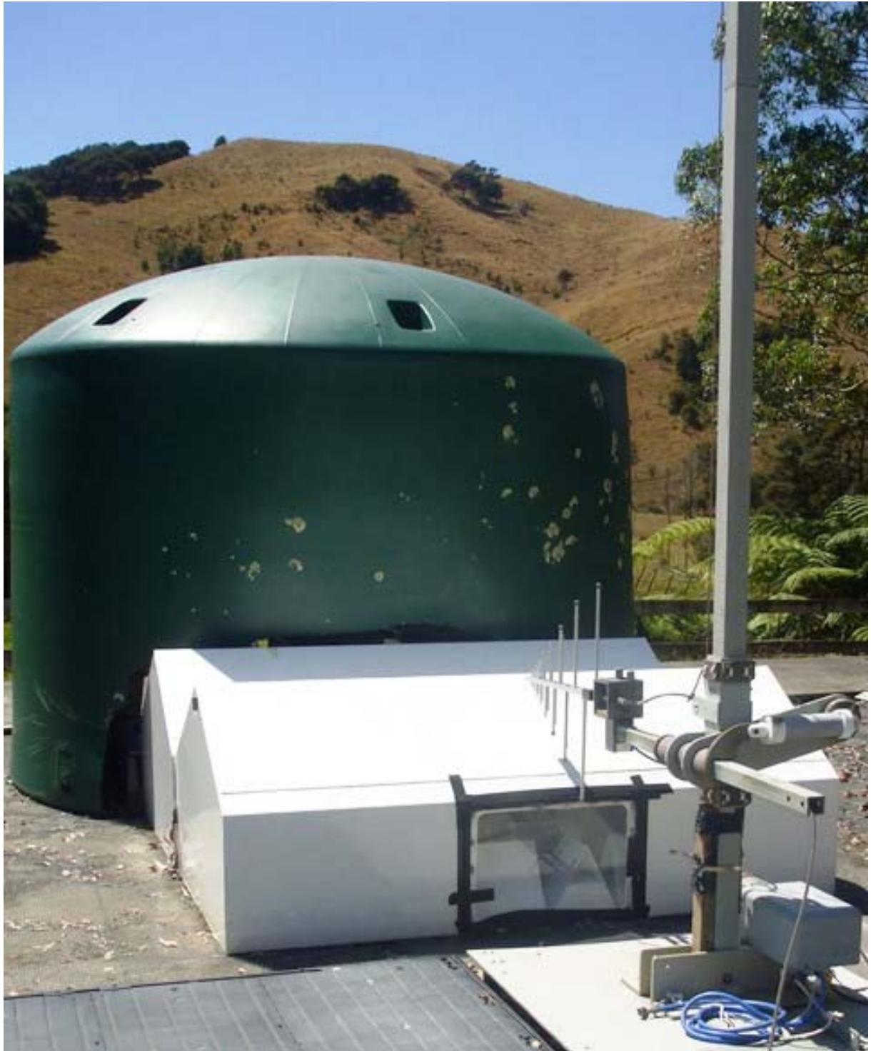
Schwarzbeck log periodic antenna (300 – 1000 MHz)
