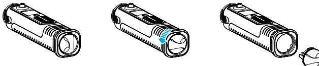
To detach, turn the cap on the S1 Handle counter-clockwise.
