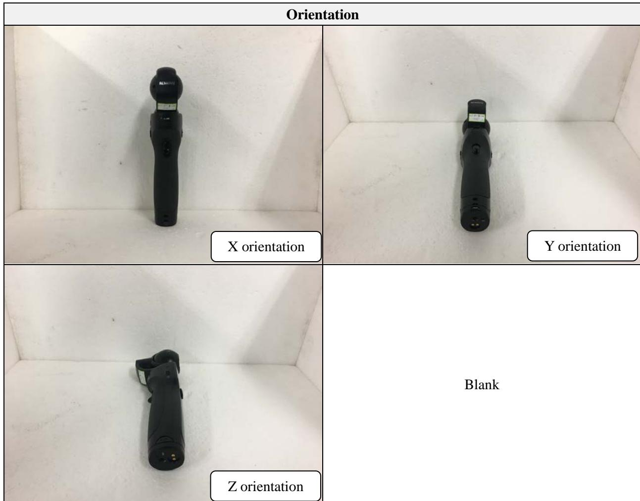
Note. : Radiated testing was performed with the EUT in worst-case X orientation.
