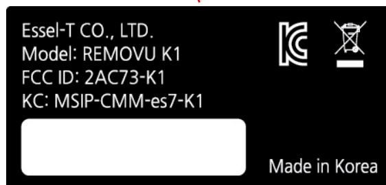
The device is so small that it is not practicable to place the statement specified under 15.19 statement request, the information required by this paragraph shall be placed in a Prominent location in the User's Manual.
