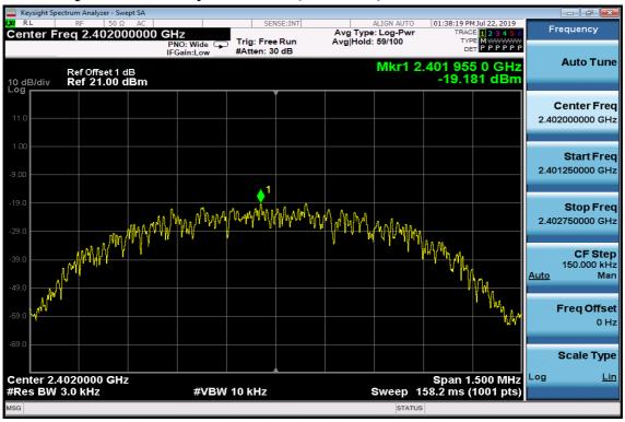
**Power Spectral Density Test Plot (CH-Mid)**
