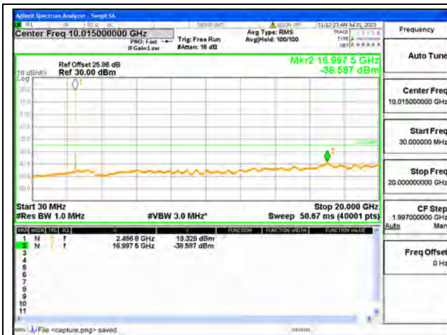
B41-30M-20G / 20MHz / Low CH / QPSK
