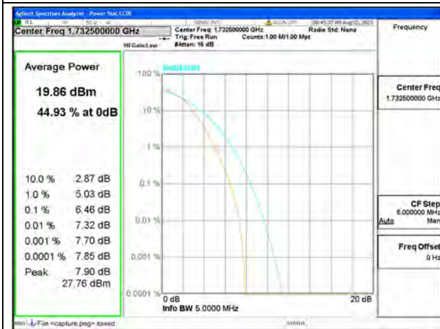
B4 / 5MHz / Mid CH / 16QAM
