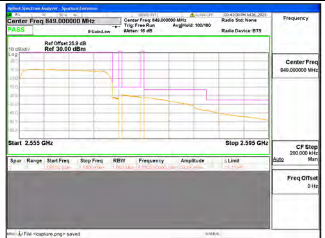
B7 / 15MHz / High CH / QPSK / FULL RB
