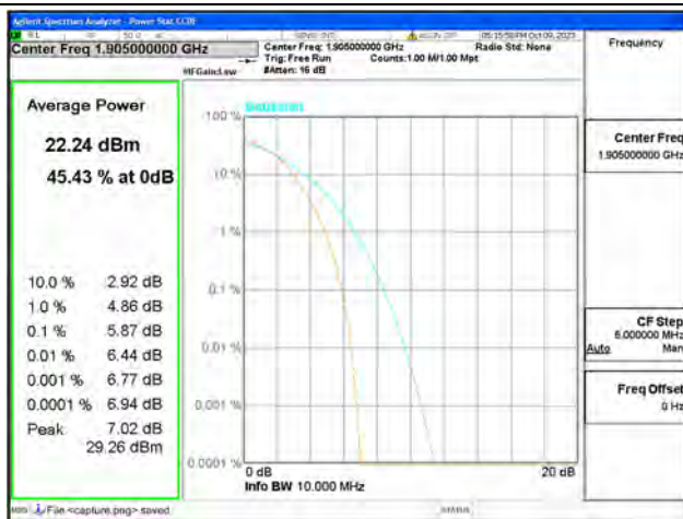
B2 / 10MHz / High CH / 16QAM
