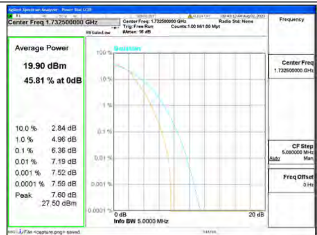
B4 / 1.4MHz / Mid CH / 64QAM
