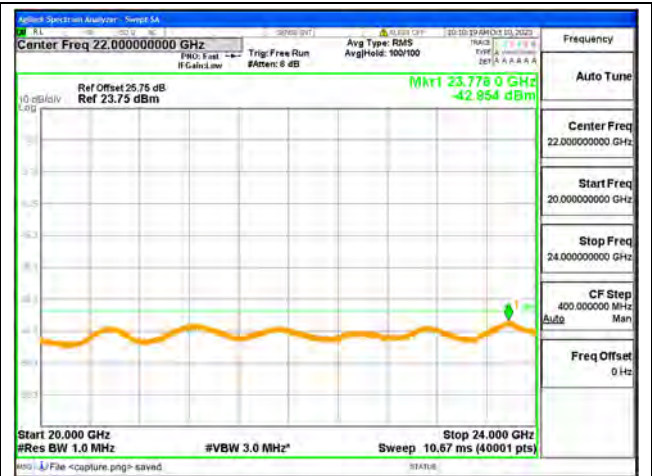
B40-2-20G-24G / 5MHz / High CH / QPSK
