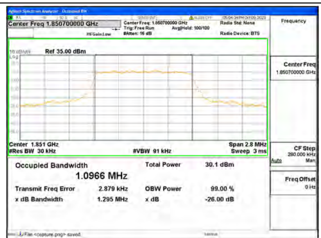
B2 / 1.4MHz / 16QAM/ Low CH
