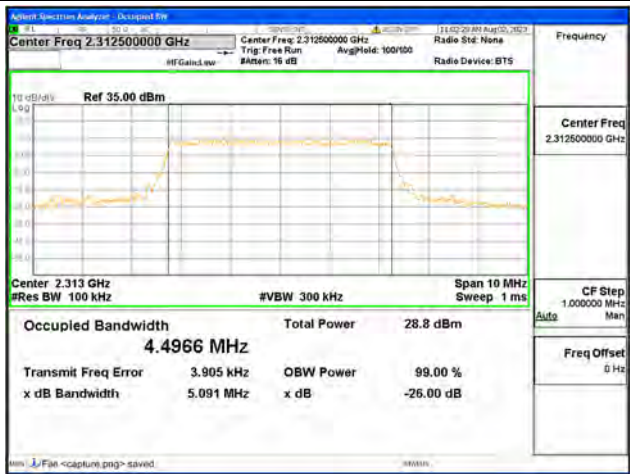
B40-1 / 5MHz / 64QAM/ High CH
