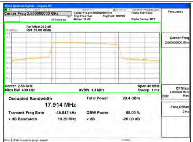
B7 / 20MHz / 64QAM/ High CH
