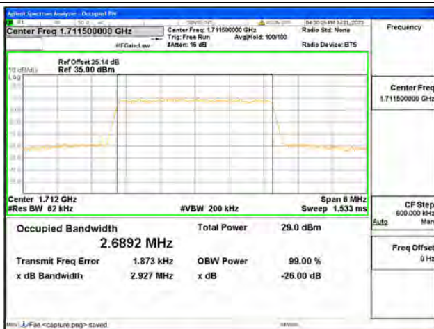
B4 / 3MHz / 16QAM/ Low CH
