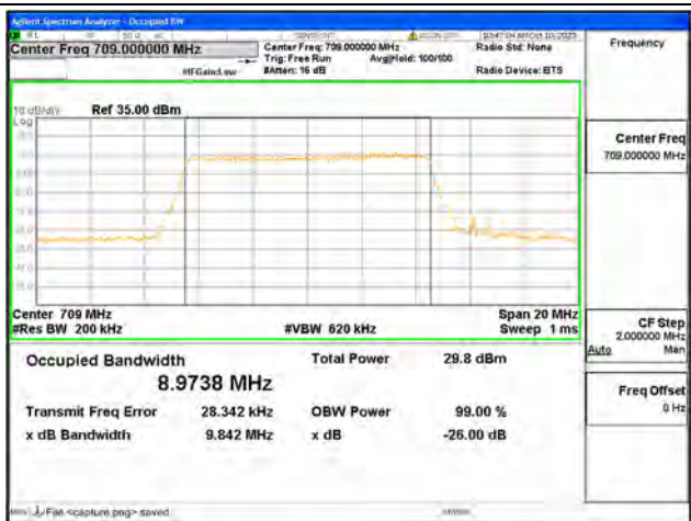
B17 / 10MHz / 16QAM/ Low CH
