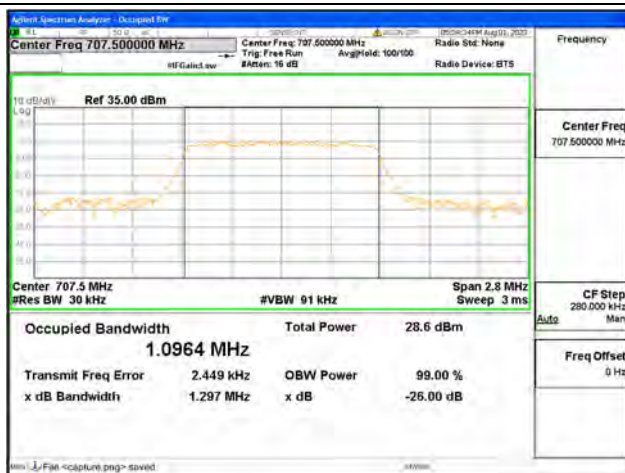
B12 / 1.4MHz / 16QAM/ Mid CH
