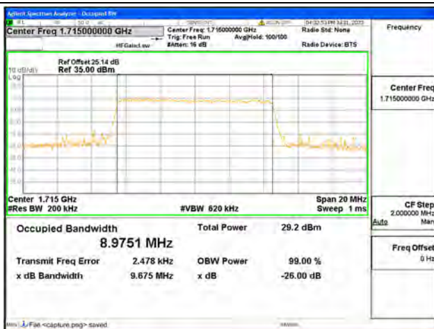
B4 / 10MHz / 16QAM/ Low CH
