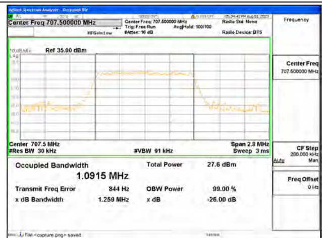
B12 / 1.4MHz / 64QAM/ Mid CH
