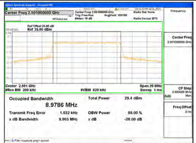
B41 / 10MHz / 64QAM/ Low CH
