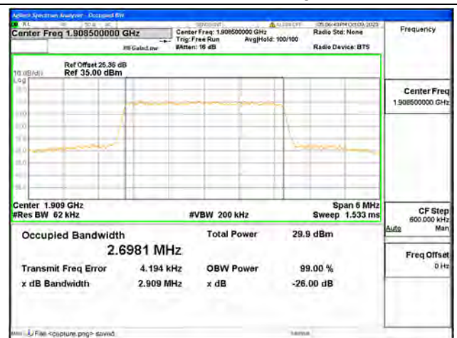
B2 / 3MHz / 64QAM / High CH
