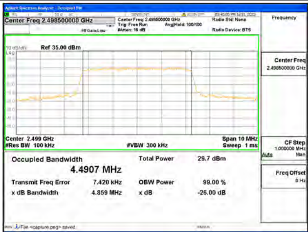
B41 / 5MHz / 64QAM/ Low CH
