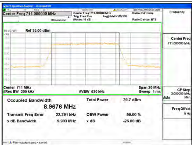
B17 / 10MHz / 16QAM/ High CH
