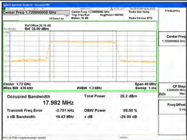
B4 / 20MHz / 16QAM/ Low CH
