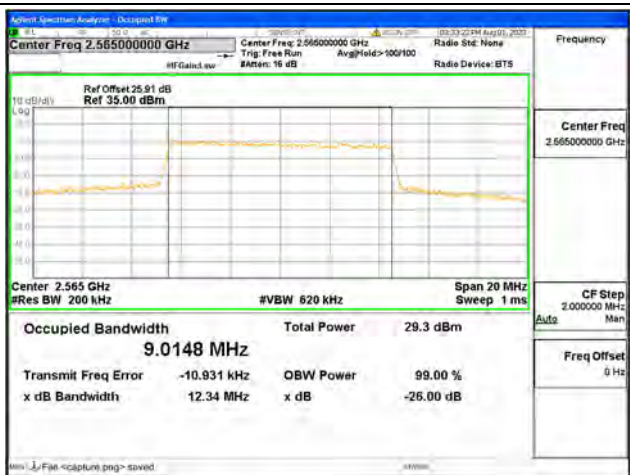
B7 / 10MHz / 16QAM/ High CH
