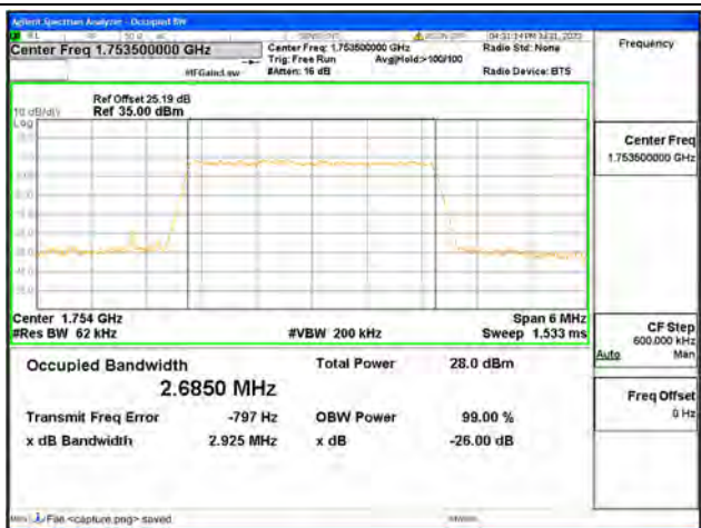
B4 / 3MHz / 16QAM / High CH
