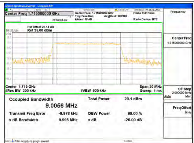
B4 / 10MHz / 64QAM/ Low CH
