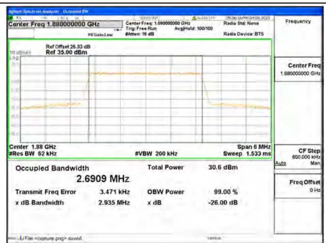
B2 / 3MHz / 16QAM / Mid CH
