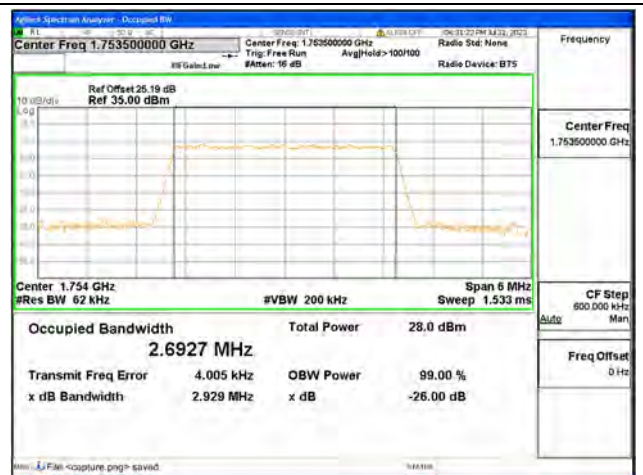
B4 / 3MHz / 64QAM / High CH
