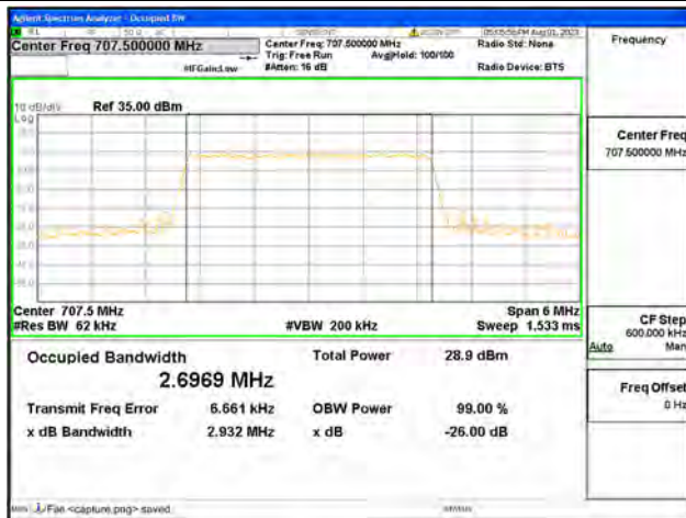
B12 / 3MHz / 64QAM/ Mid CH
