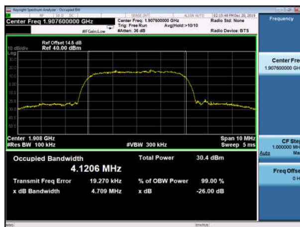
(Plot F3: WCDMA 1900MHz Channel = 9538 Occupied bandwidth)
