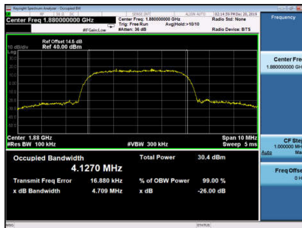
(Plot F2: WCDMA 1900MHz Channel = 9400 Occupied bandwidth)
