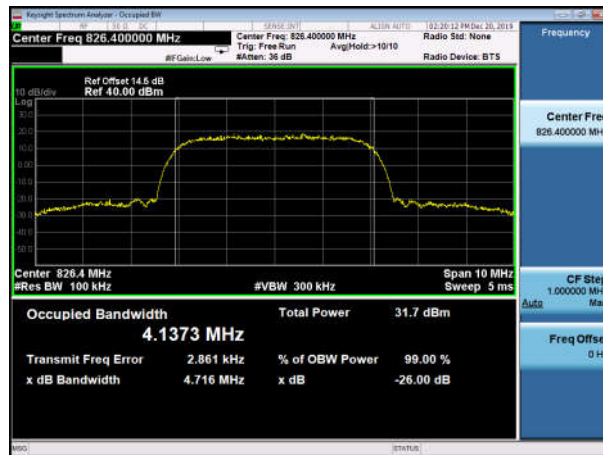
(Plot E1: WCDMA 850MHz Channel = 4132 Occupied bandwidth)
