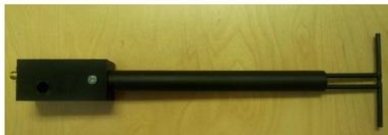
Figure 1 – MVG COMOSAR Validation Dipole
