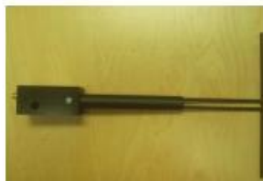
Figure 1 – MVG COMOSAR Validation Dipole
