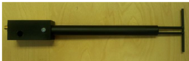
Figure 1 – MVG COMOSAR Validation Dipole
