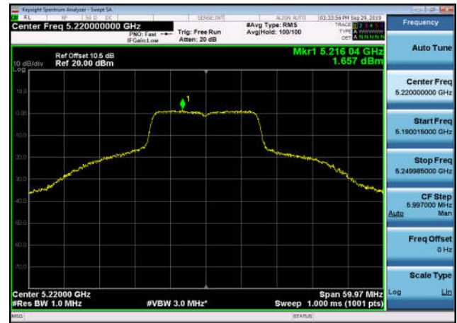
U-NII-1 Power spectral density-802.11 n(40MHz),5190MHz,Ant1
