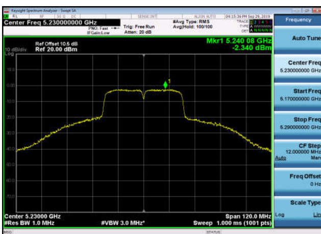
U-NII-1 Power spectral density-802.11 n(40MHz),5230MHz,Ant1
