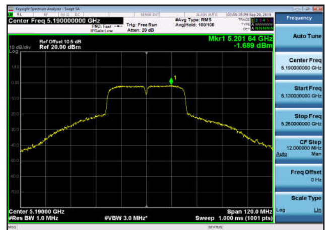
U-NII-1 Power spectral density-802.11 a(20MHz),5180MHz,Ant1
