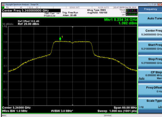
U-NII-1 Power spectral density-802.11 n(40MHz),5230MHz,Ant1
