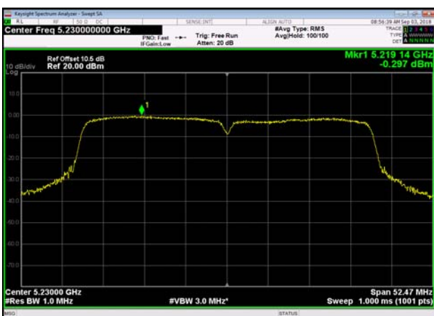
U-NII-1 Power spectral density-802.11 n(40MHz),5230MHz
