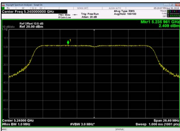
U-NII-1 Power spectral density-802.11 n(40MHz),5230MHz
