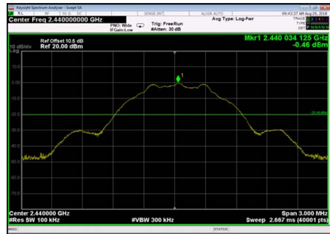
,Plot ,2 Conducted Emission: 2402 Band Edge
