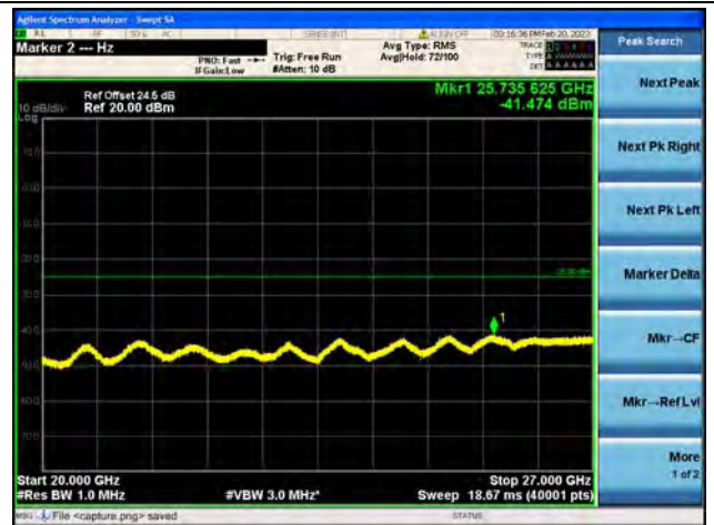
Band41(2535~2655)-20G-27G / 15MHz / High CH / 16QAM
