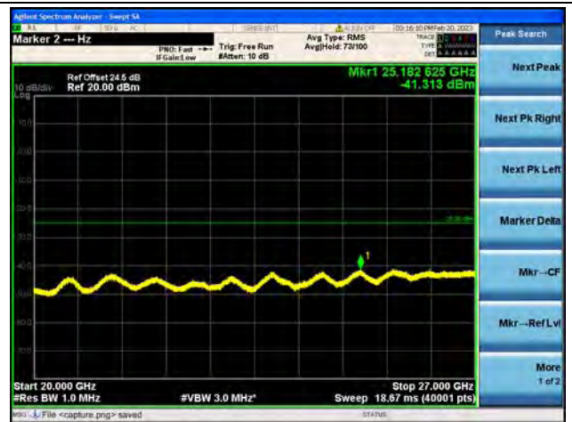
Band41(2535~2655)-20G-27G / 15MHz / High CH / QPSK
