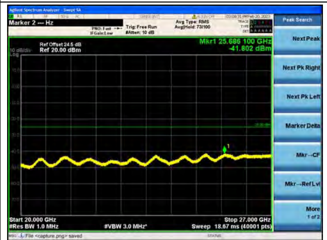
Band41(2535~2655)-20G-27G / 5MHz / High CH / 16QAM
