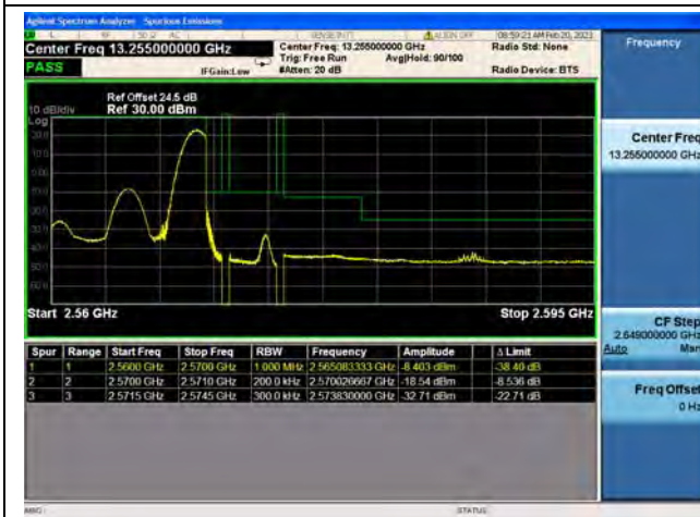
Band7 / 10MHz / High CH / QPSK / 1 RB
