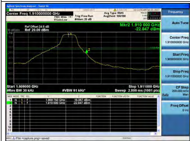
Band2 / 3MHz / High CH / QPSK / 1 RB
