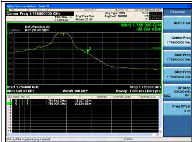
Band4 / 5MHz / High CH / QPSK / 1 RB
