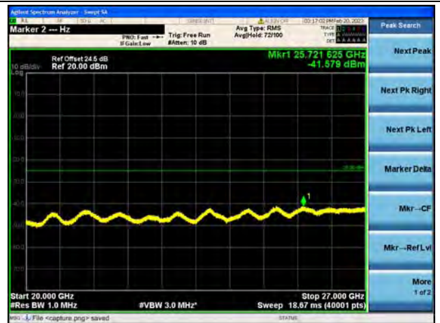
Band41(2535~2655)-20G-27G / 15MHz / High CH / 64QAM
