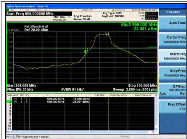
Band12 / 3MHz / Low CH / QPSK / 1 RB
