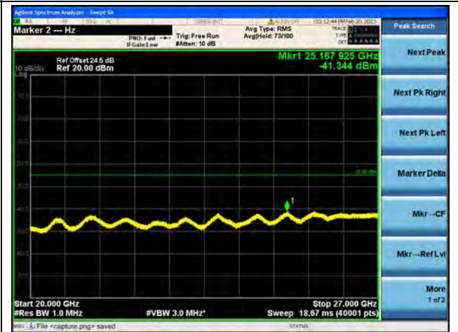
Band41(2535~2655)-20G-27G / 10MHz / High CH / 16QAM
