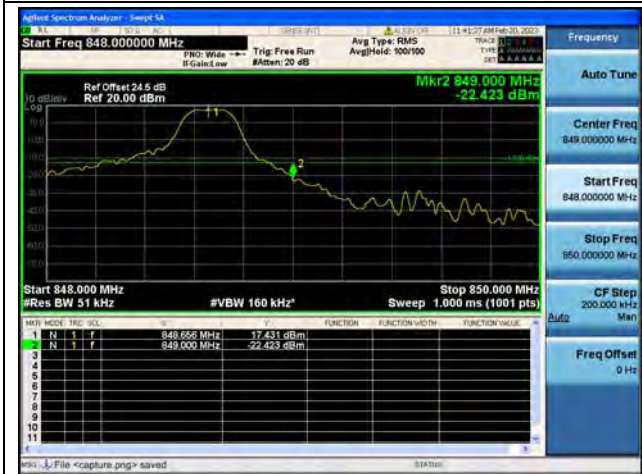
Band5 / 5MHz / High CH / QPSK / 1 RB
