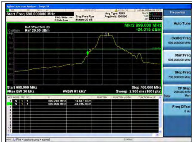
Band12 / 1.4MHz / Low CH / QPSK / 1 RB
