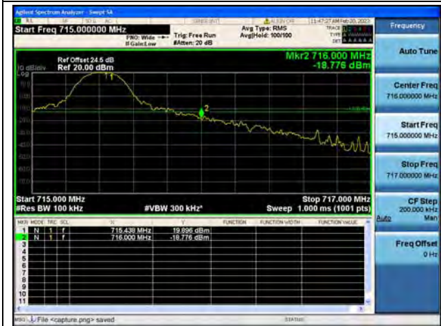
Band17 / 10MHz / High CH / QPSK / 1 RB
