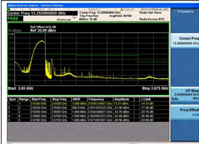
Band41 / 10MHz / High CH / QPSK / 1 RB
