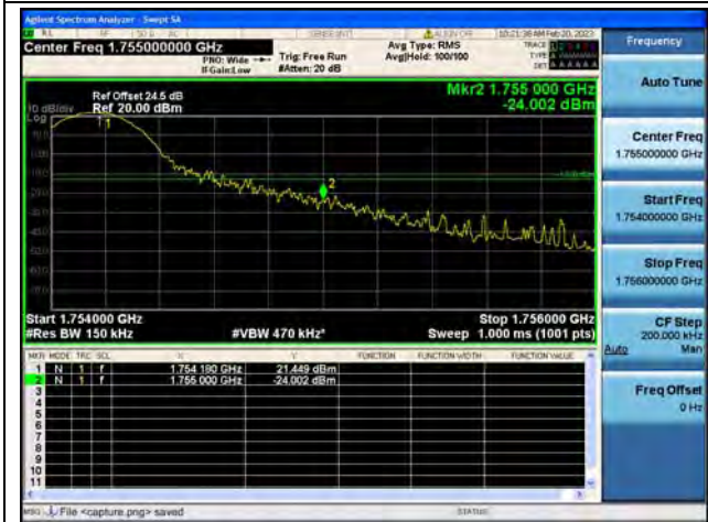
Band4 / 15MHz / High CH / QPSK / 1 RB
