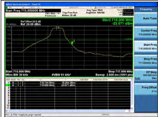
Band12 / 3MHz / High CH / QPSK / 1 RB
