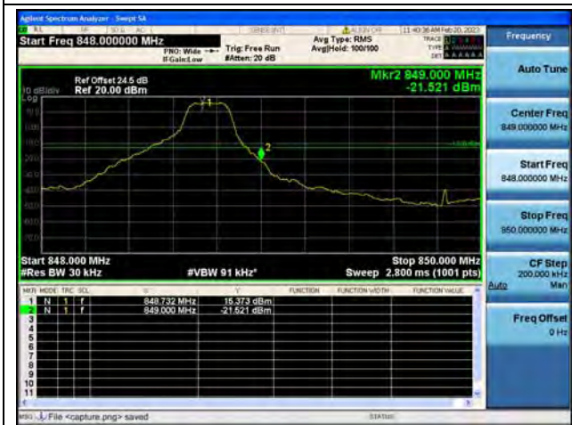
Band5 / 3MHz / High CH / QPSK / 1 RB
