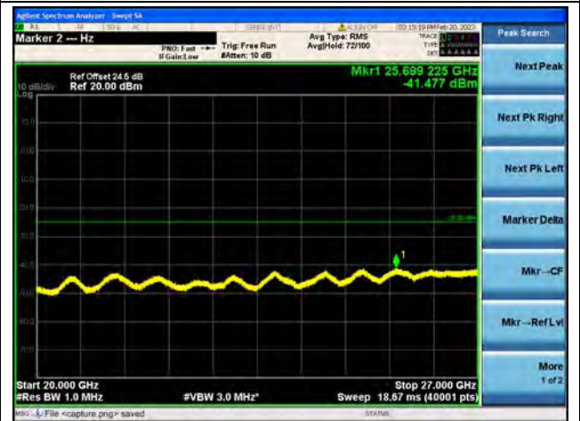
Band41(2535~2655)-20G-27G / 15MHz / Mid CH / 16QAM
