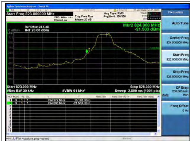
Band5 / 3MHz / Low CH / QPSK / 1 RB
