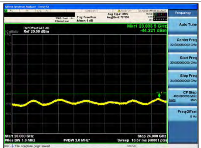
Band40-2-20G-24G / 5MHz / High CH / QPSK
