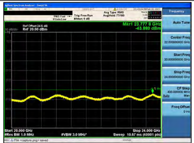
Band40-2-20G-24G / 5MHz / High CH / 16QAM
