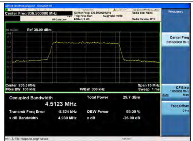
Band5 / 5MHz / 64QAM/ Mid CH
