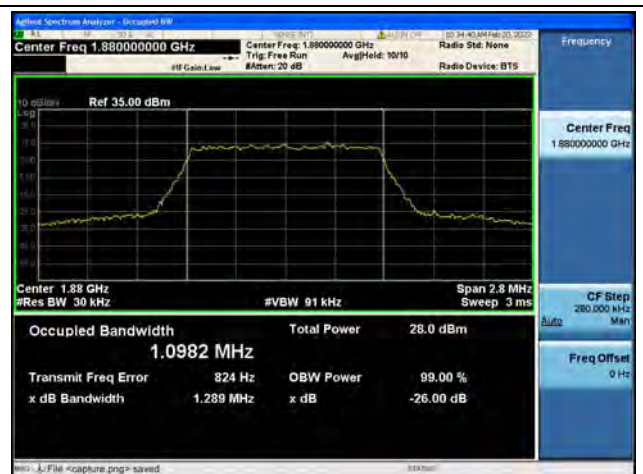
Band2 / 1.4MHz / 64QAM/ Mid CH
