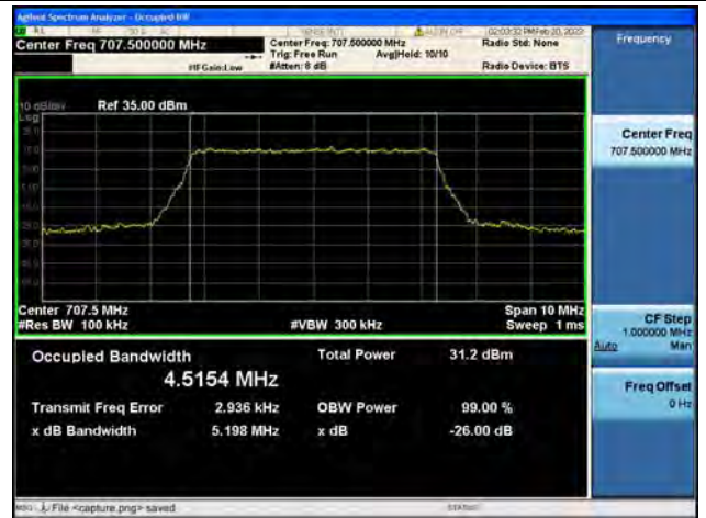
Band12 / 5MHz / QPSK/ Mid CH
