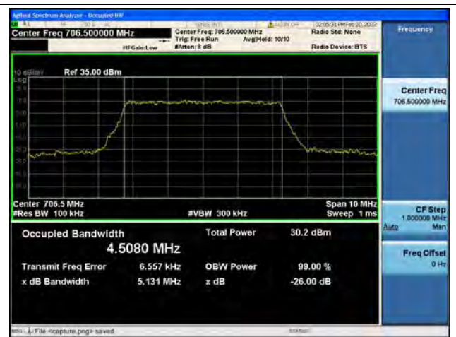
Band17 / 5MHz / 16QAM/ Low CH
