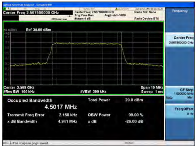
Band7 / 5MHz / 64QAM / High CH
