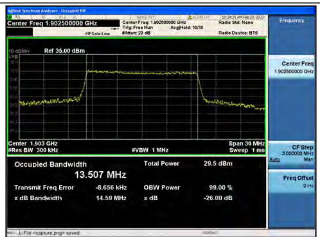
Band2 / 15MHz / 16QAM/ High CH
