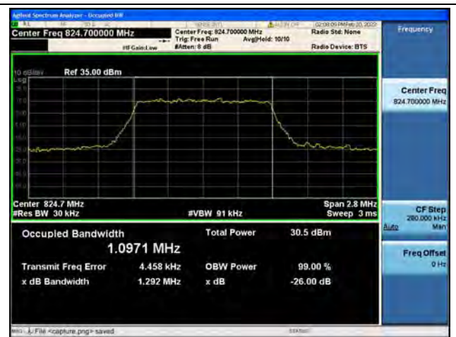
Band5 / 1.4MHz / 16QAM/ Low CH
