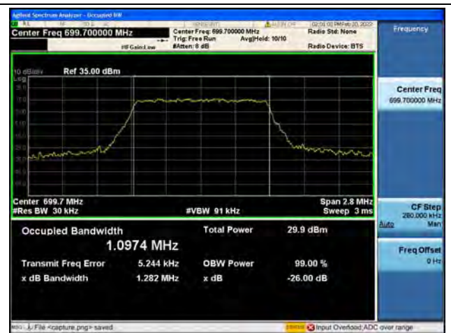
Band12 / 1.4MHz / 16QAM/ Low CH
