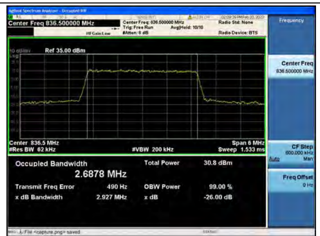
Band5 / 3MHz / 16QAM/ Mid CH
