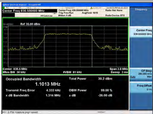
Band5 / 1.4MHz / 16QAM/ Mid CH
