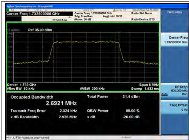
Band4 / 3MHz / QPSK/ Mid CH
