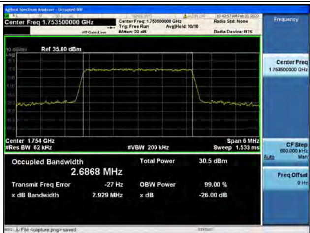
Band4 / 3MHz / 16QAM/ High CH
