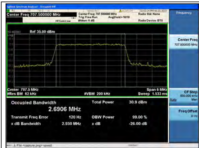
Band12 / 3MHz / QPSK/ Mid CH
