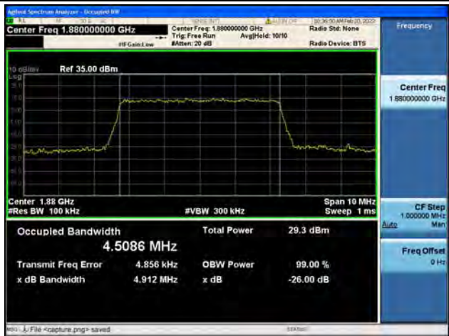
Band2 / 5MHz / 16QAM/ Mid CH
