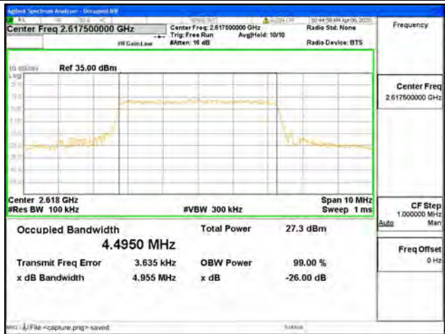
Band38 / 5MHz / 64QAM/ High CH
