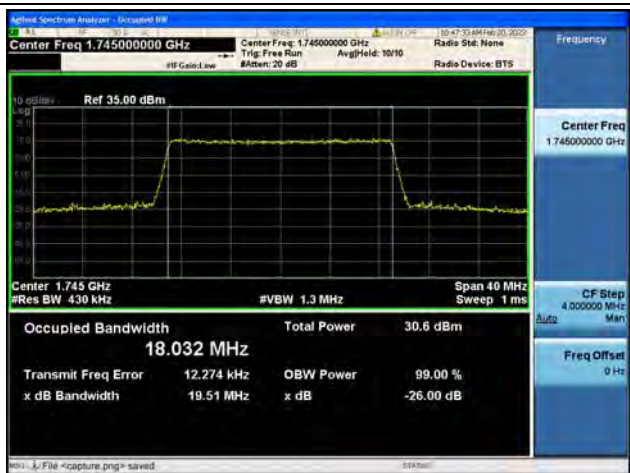
Band4 / 20MHz / 16QAM/ High CH
