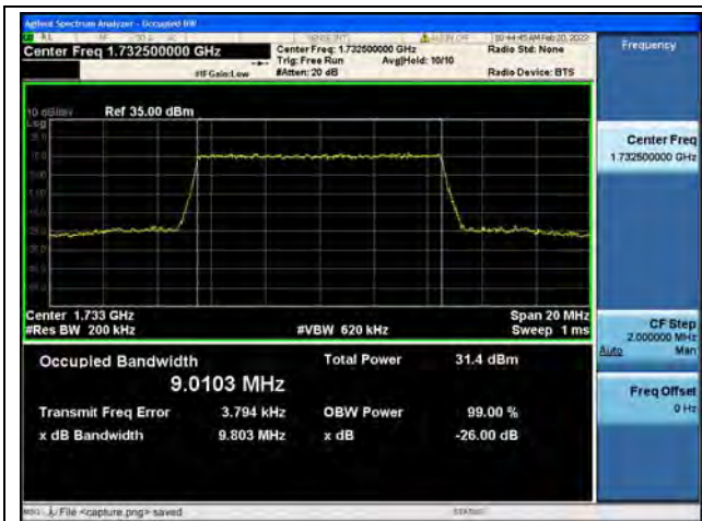
Band4 / 10MHz / QPSK/ Mid CH
