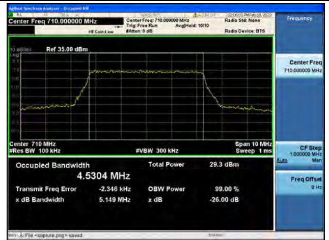
Band17 / 5MHz / 64QAM/ Mid CH
