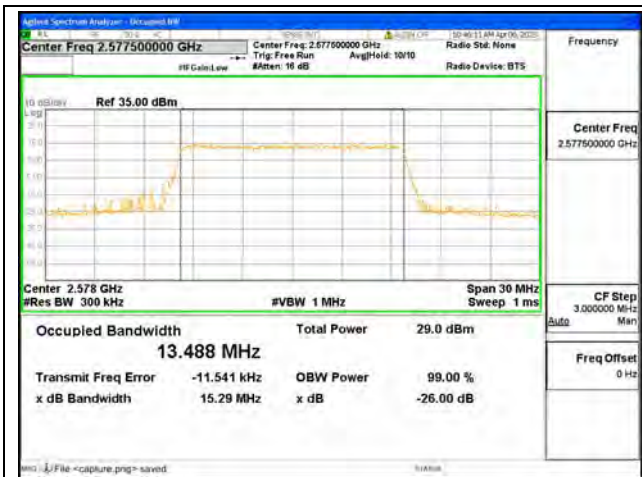
Band38 / 15MHz / QPSK / Low CH
