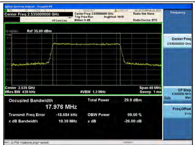
Band7 / 20MHz / 16QAM/ Mid CH
