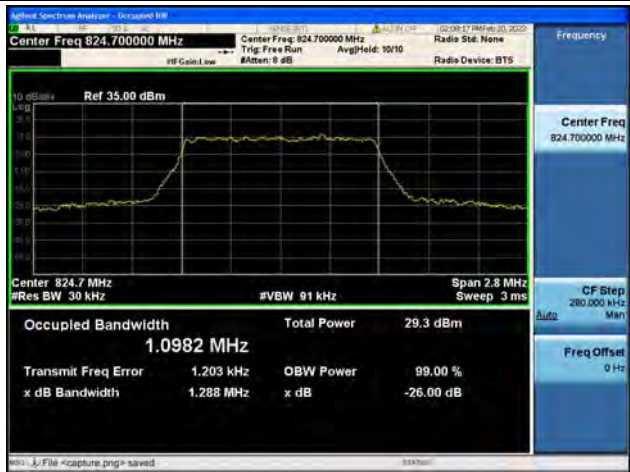
Band5 / 1.4MHz / 64QAM/ Low CH
