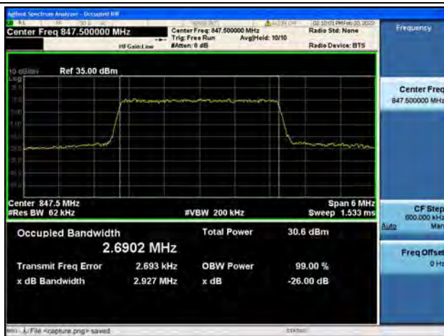
Band5 / 3MHz / 16QAM/ High CH
