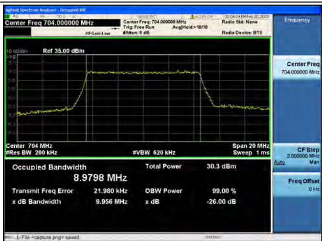
Band12 / 10MHz / 16QAM/ Low CH
