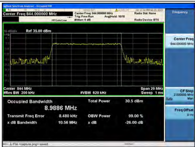
Band5 / 10MHz / 16QAM/ High CH
