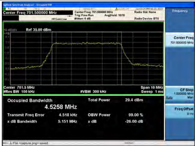
Band12 / 5MHz / 64QAM/ Low CH
