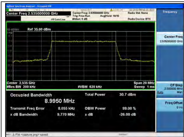
Band7 / 10MHz / QPSK/ Mid CH
