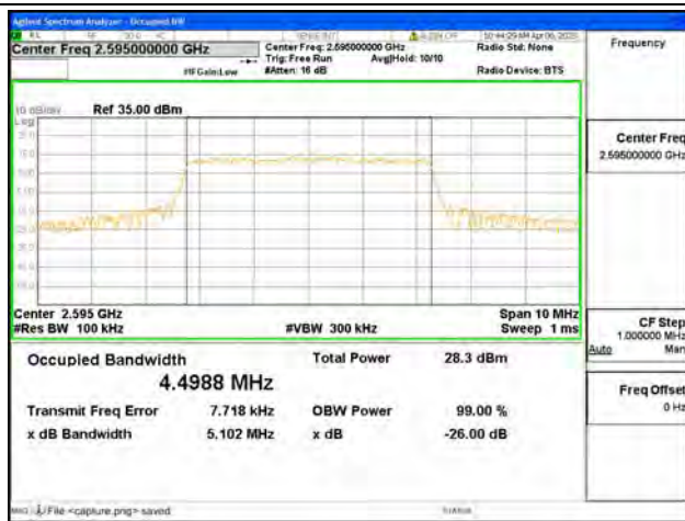
Band38 / 5MHz / 16QAM/ Mid CH
