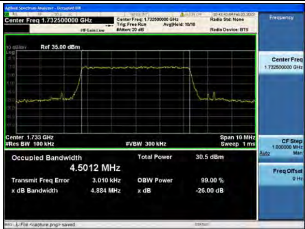
Band4 / 5MHz / 16QAM/ Mid CH
