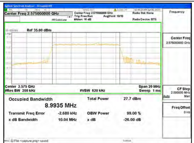
Band38 / 10MHz / 64QAM/ Low CH
