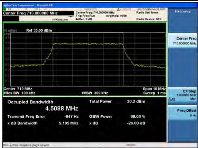
Band17 / 5MHz / 16QAM/ Mid CH
