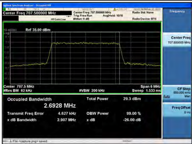
Band12 / 3MHz / 64QAM/ Mid CH
