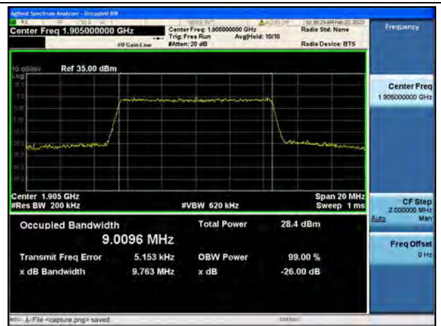
Band2 / 10MHz / 64QAM/ High CH
