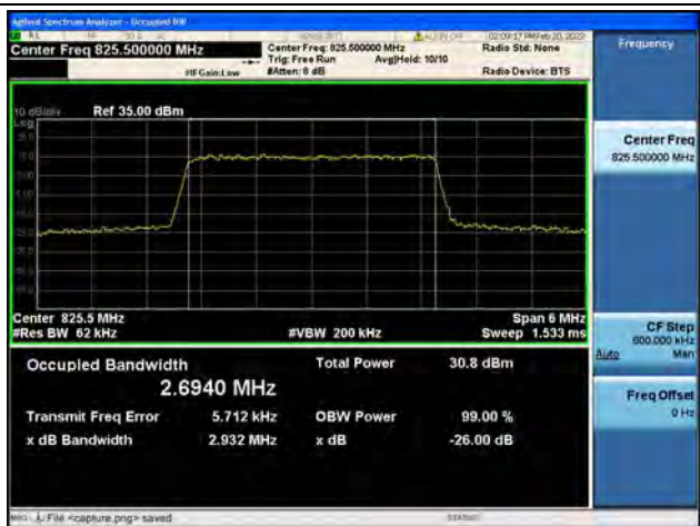
Band5 / 3MHz / 16QAM/ Low CH
