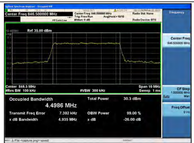
Band5 / 5MHz / 16QAM / High CH
