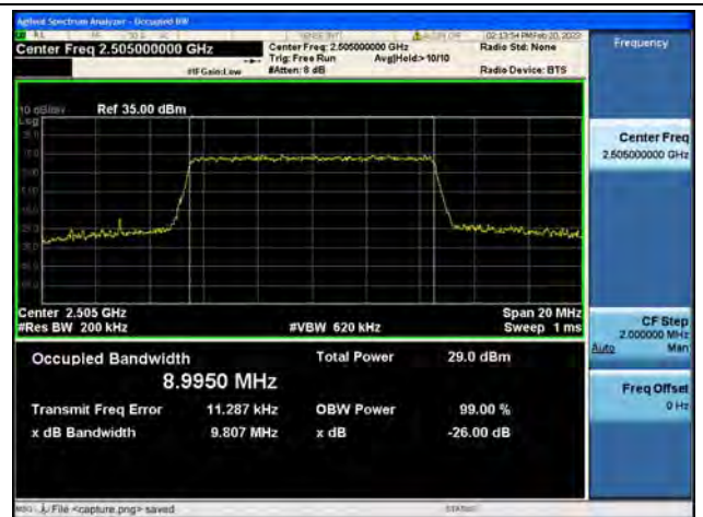
Band7 / 10MHz / 64QAM / Low CH
