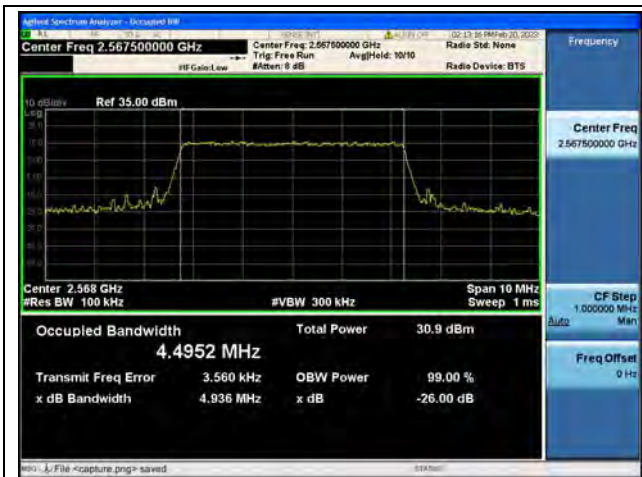
Band7 / 5MHz / QPSK / High CH
