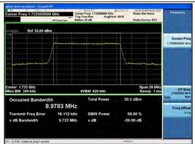
Band4 / 10MHz / 16QAM/ Mid CH
