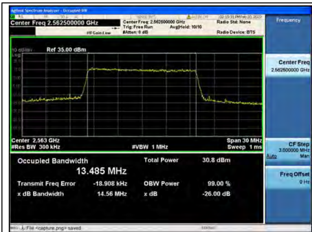
Band7 / 15MHz / QPSK/ High CH
