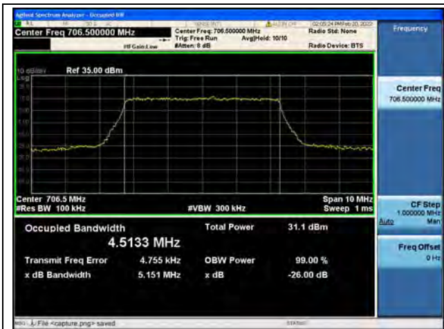
Band17 / 5MHz / QPSK/ Low CH
