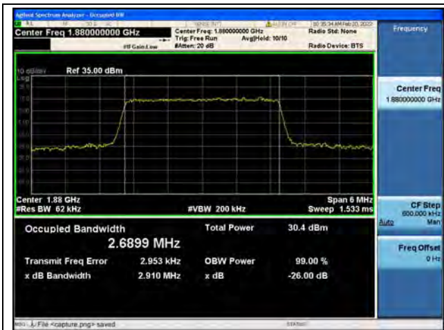
Band2 / 3MHz / QPSK/ Mid CH
