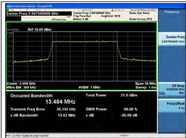
Band7 / 15MHz / QPSK/ Low CH
