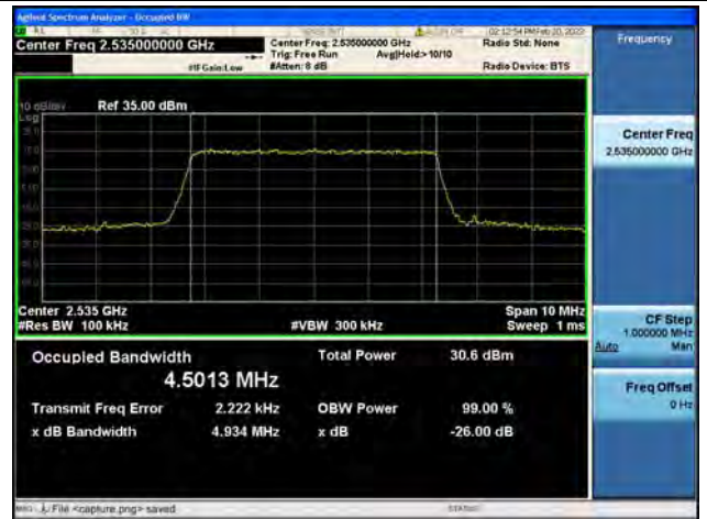
Band7 / 5MHz / QPSK/ Mid CH
