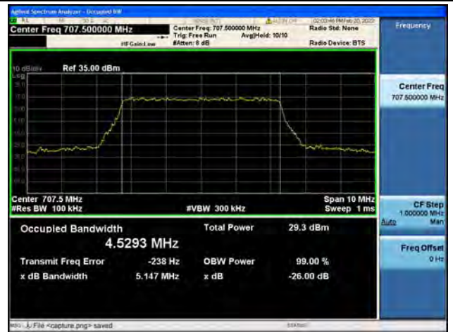
Band12 / 5MHz / 64QAM/ Mid CH
