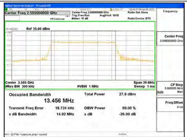
Band38 / 15MHz / 64QAM / Mid CH
