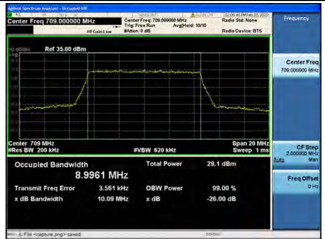
Band17 / 10MHz / 64QAM/ Low CH
