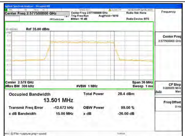
Band38 / 15MHz / 16QAM / Low CH
