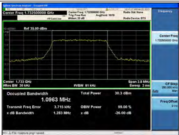
Band4 / 1.4MHz / 16QAM/ Mid CH
