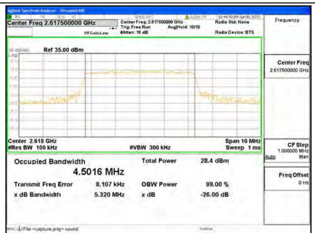
Band38 / 5MHz / 16QAM/ High CH
