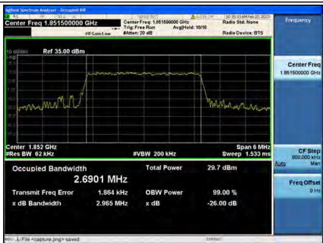
Band2 / 3MHz / 16QAM/ Low CH
