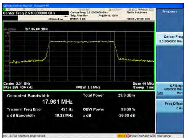
Band7 / 20MHz / 16QAM/ Low CH
