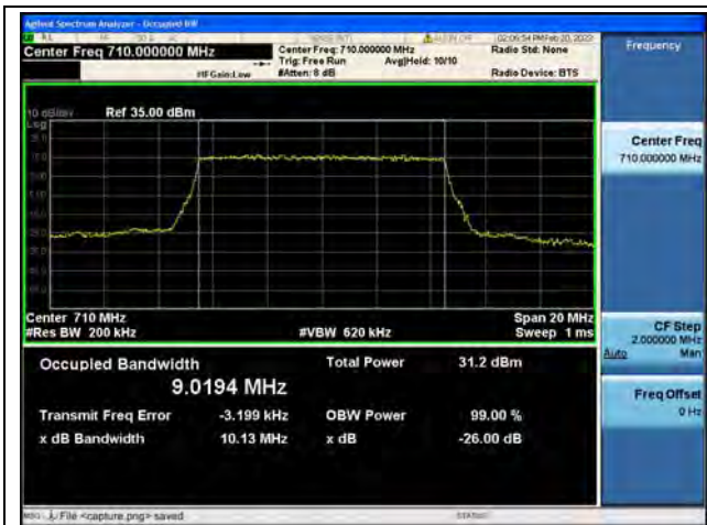
Band17 / 10MHz / QPSK/ Mid CH
