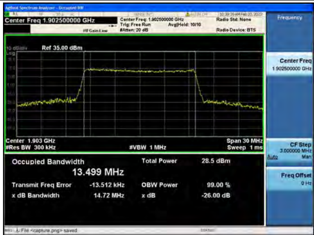
Band2 / 15MHz / 64QAM/ High CH
