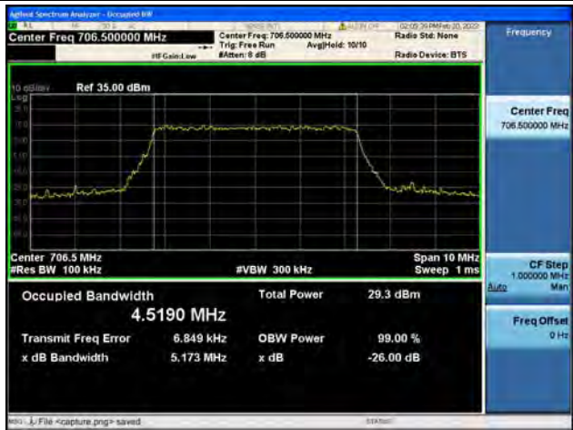
Band17 / 5MHz / 64QAM/ Low CH
