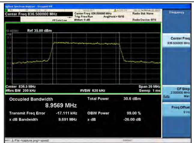
Band5 / 10MHz / 16QAM/ Mid CH
