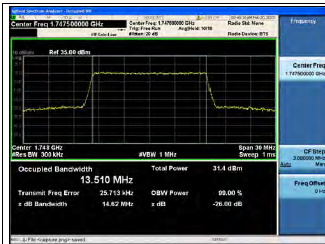
Band4 / 15MHz / QPSK/ High CH
