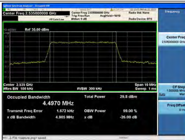
Band7 / 5MHz / 16QAM/ Mid CH
