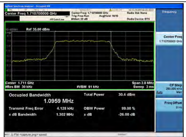
Band4 / 1.4MHz / 16QAM/ Low CH
