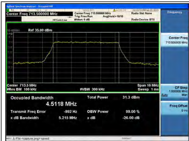
Band12 / 5MHz / QPSK/ High CH
