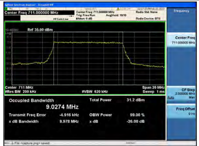
Band17 / 10MHz / QPSK/ High CH
