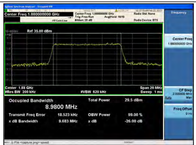
Band2 / 10MHz / 16QAM/ Mid CH
