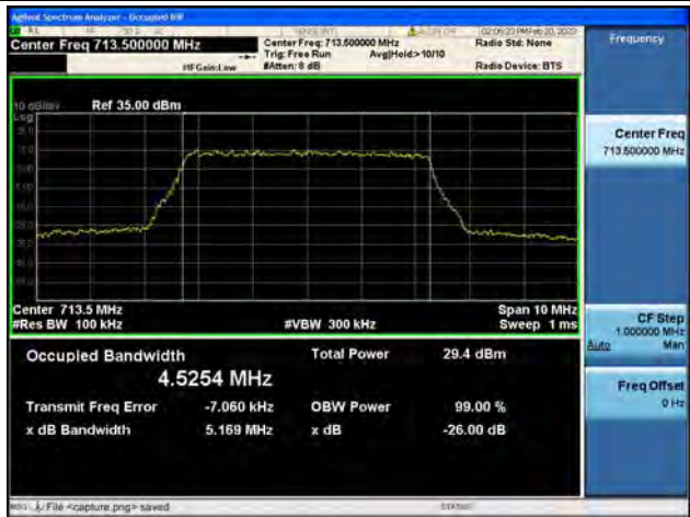
Band17 / 5MHz / 64QAM/ High CH
