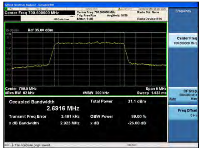
Band12 / 3MHz / QPSK/ Low CH
