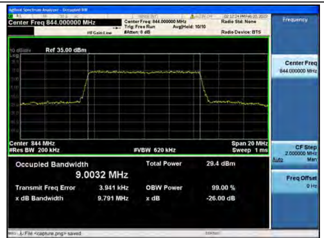
Band5 / 10MHz / 64QAM/ High CH
