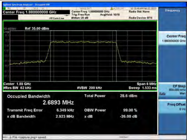
Band2 / 3MHz / 64QAM/ Mid CH
