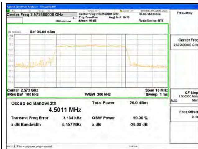
Band38 / 5MHz / QPSK/ Low CH
