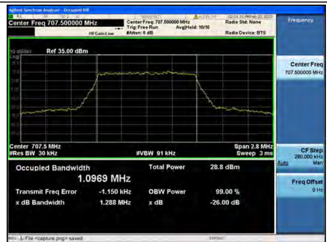
Band12 / 1.4MHz / 64QAM/ Mid CH
