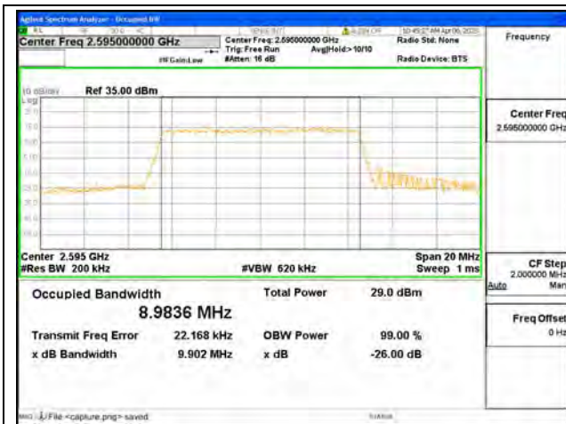
Band38 / 10MHz / QPSK/ Mid CH
