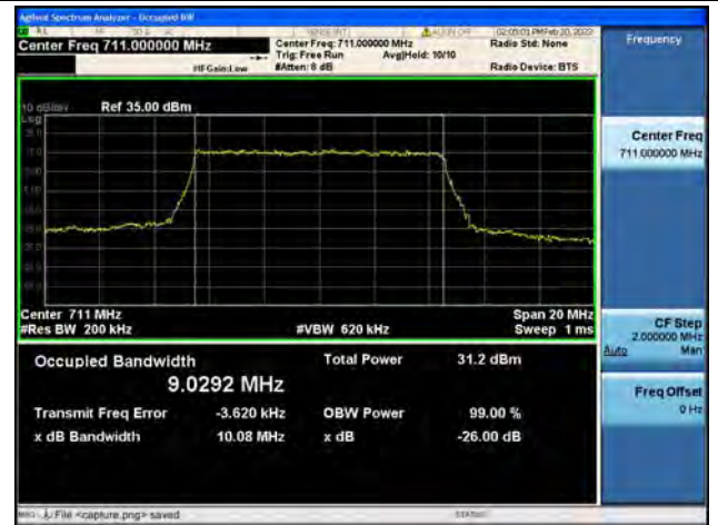
Band12 / 10MHz / QPSK/ High CH
