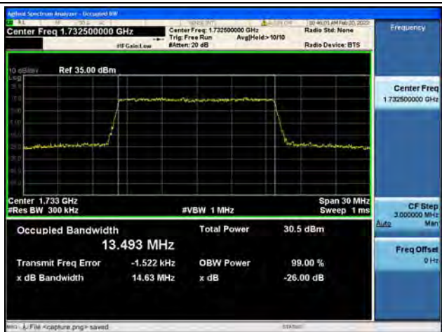
Band4 / 15MHz / 16QAM/ Mid CH
