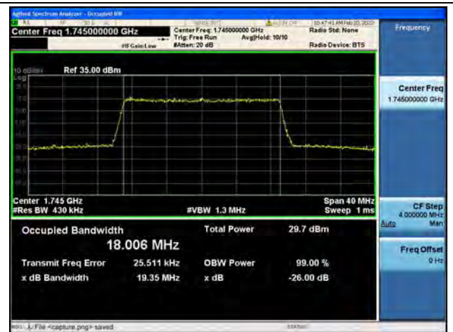
Band4 / 20MHz / 64QAM/ High CH
