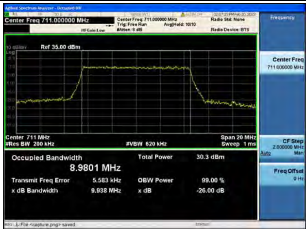
Band17 / 10MHz / 16QAM/ High CH
