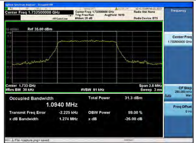
Band4 / 1.4MHz / QPSK/ Mid CH
