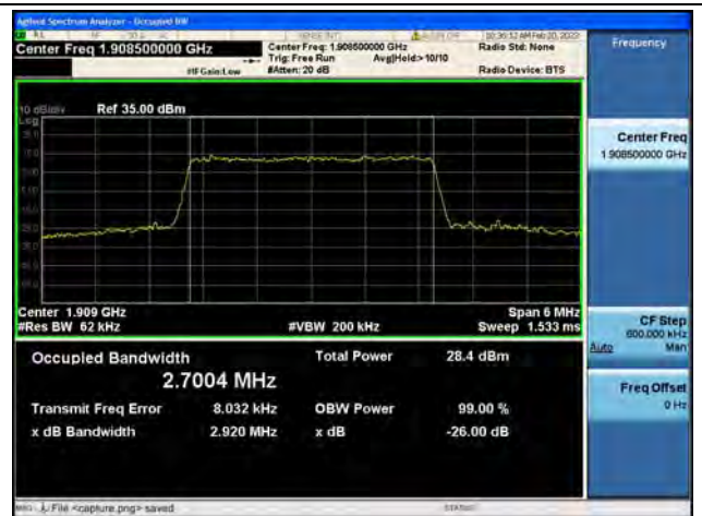
Band2 / 3MHz / 64QAM/ High CH
