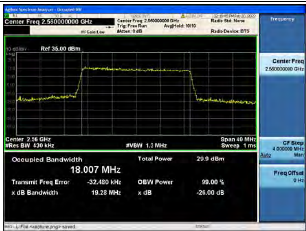
Band7 / 20MHz / 16QAM/ High CH
