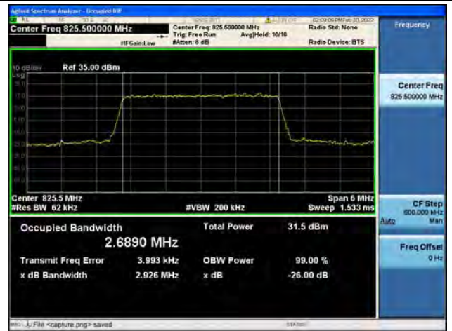
Band5 / 3MHz / QPSK/ Low CH
