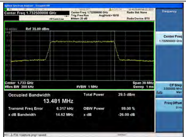
Band4 / 15MHz / 64QAM/ Mid CH
