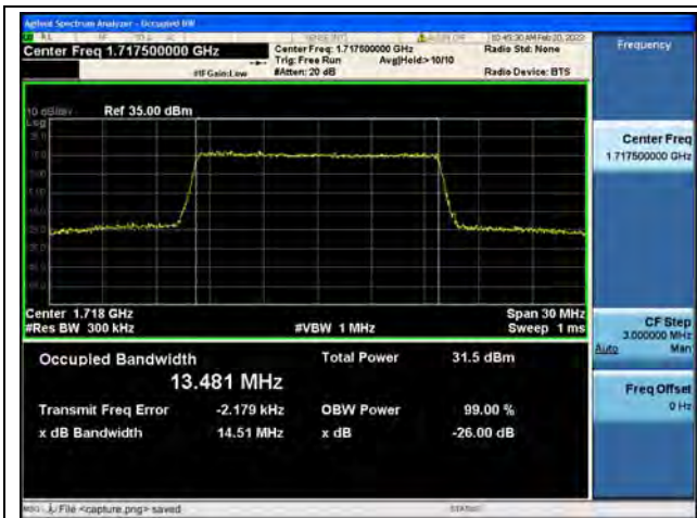
Band4 / 15MHz / QPSK/ Low CH
