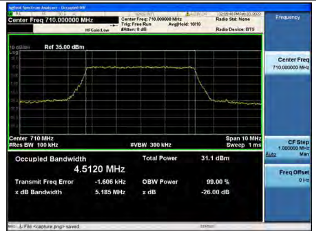
Band17 / 5MHz / QPSK/ Mid CH
