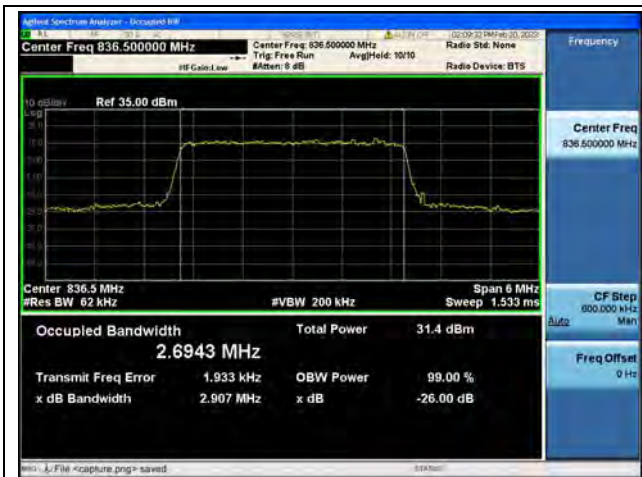
Band5 / 3MHz / QPSK/ Mid CH
