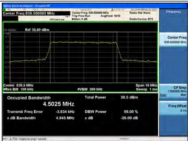
Band5 / 5MHz / 16QAM/ Mid CH
