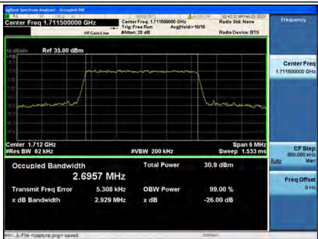
Band4 / 3MHz / 16QAM/ Low CH
