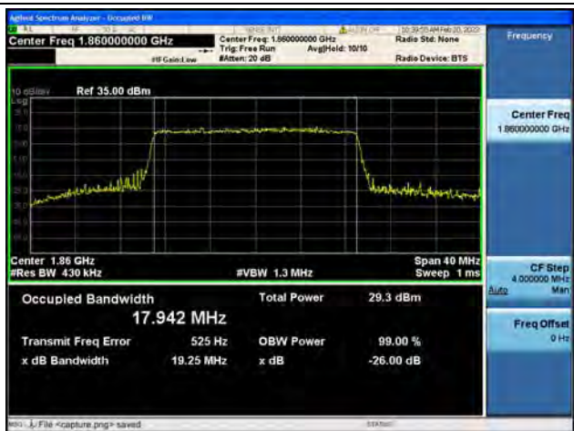
Band2 / 20MHz / 16QAM/ Low CH
