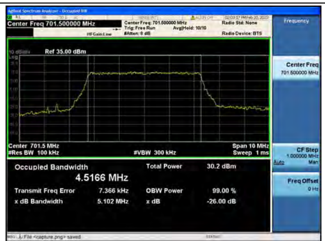
Band12 / 5MHz / 16QAM/ Low CH
