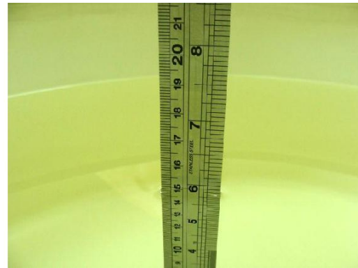
Fig 7.2 Photo of Liquid Height for Body SAR
