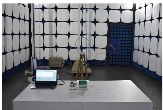
3. Radiated emission (9KHz-30MHz)
