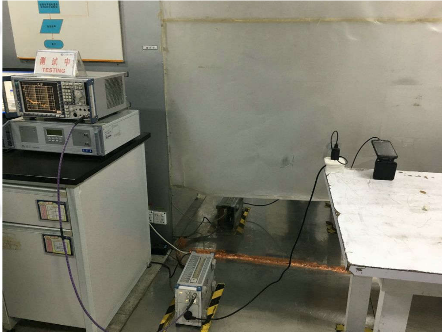
Conducted Emissions Test Setup
