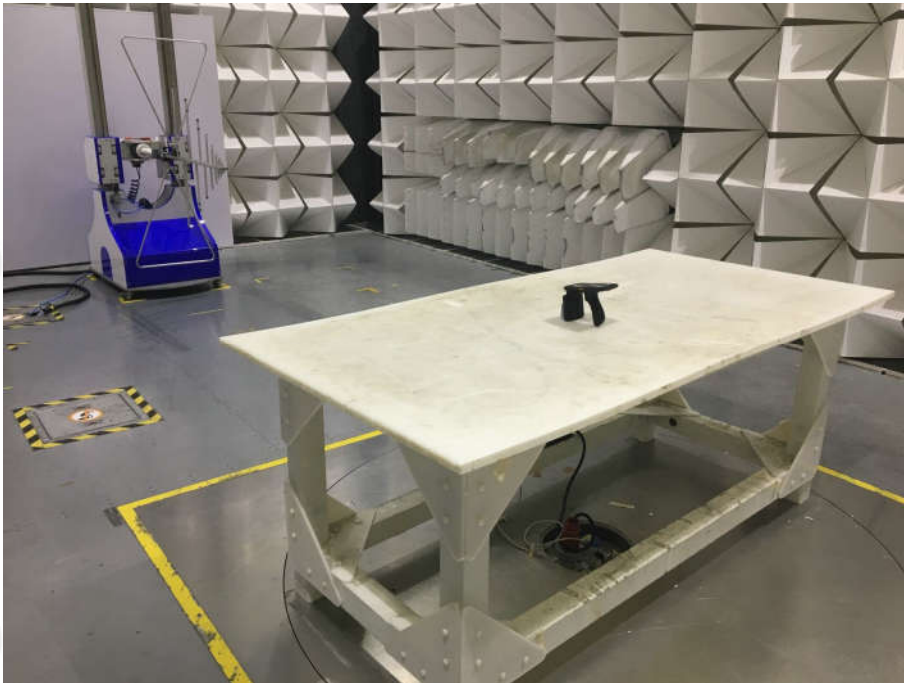
Radiated emission Test Setup (30MHz~1000MHz)
