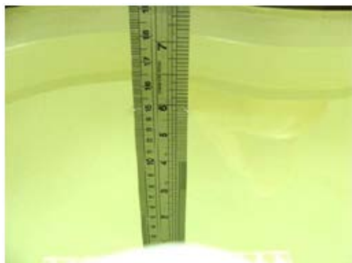
Fig 5.1 Photo of Liquid Height for Head SAR
