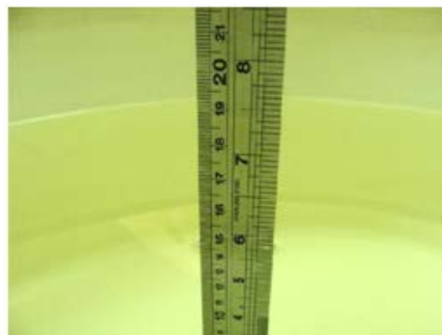
Fig 5.2 Photo of Liquid Height for Body SAR
