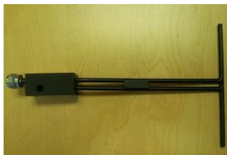
Figure 1 – MVG COMOSAR Validation Dipole
