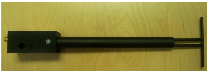
Figure 1 – MVG COMOSAR Validation Dipole
