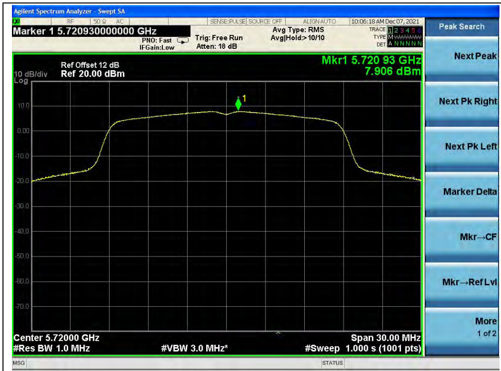
(Channel 144, 5720MHz, 802.11ac (VHT20))
