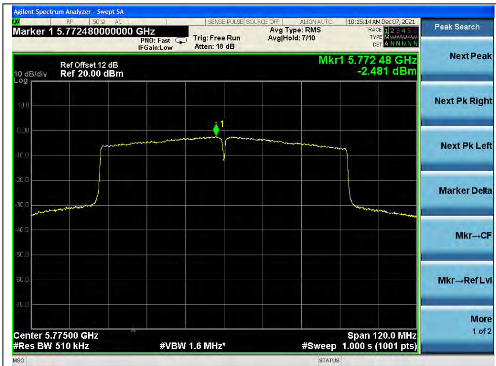
(Channel 155, 5775MHz, 802.11ac (VHT80))
