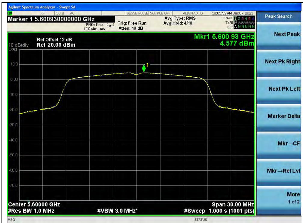
(Channel 120, 5600MHz, 802.11ac (VHT20))
