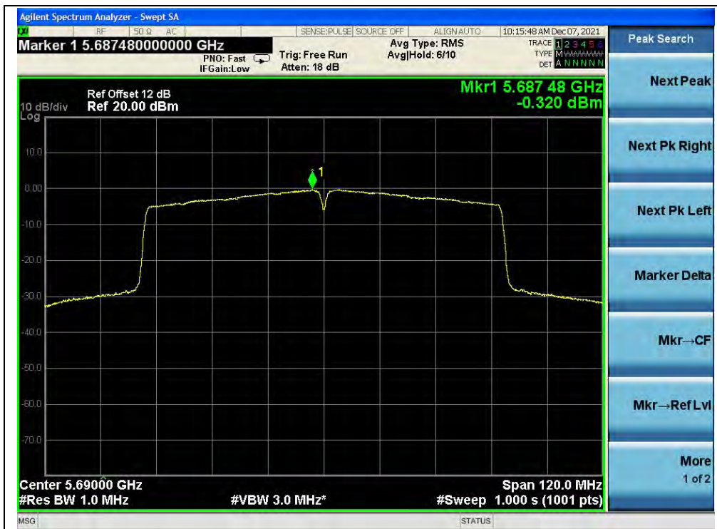
(Channel 138, 5690MHz, 802.11ac (VHT80))
