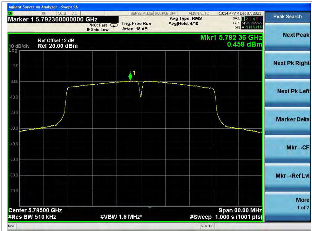
(Channel 159, 5795MHz, 802.11ac (VHT40))
