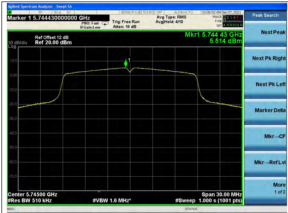
(Channel 149, 5745MHz, 802.11ac (VHT20))
