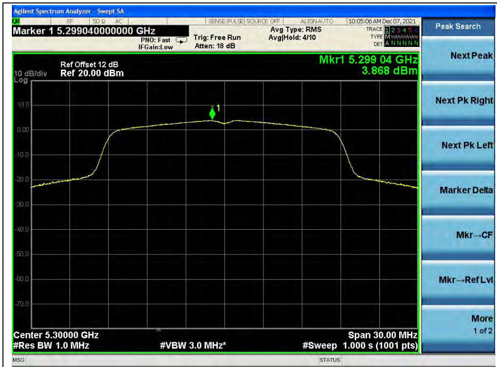
(Channel 60, 5300MHz, 802.11ac (VHT20))
