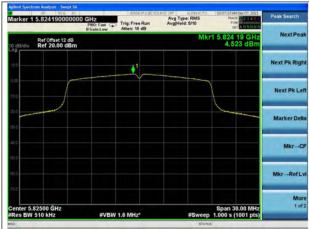
(Channel 165, 5825MHz, 802.11ac (VHT20))
