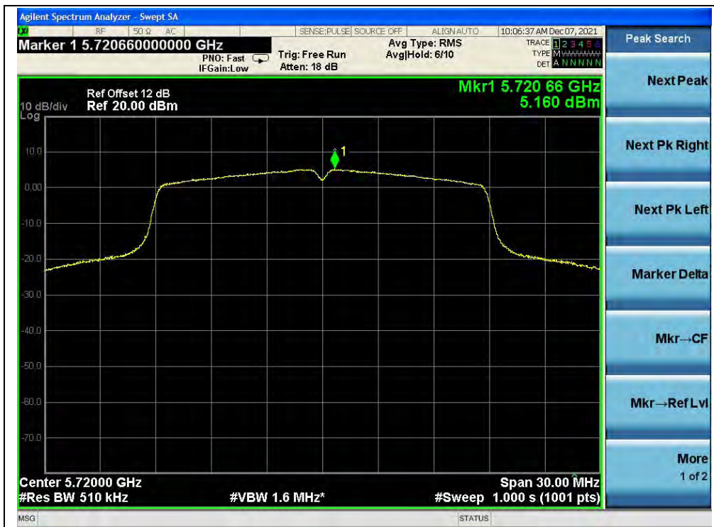
(Channel 144, 5720MHz, 802.11ac(VHT20))
