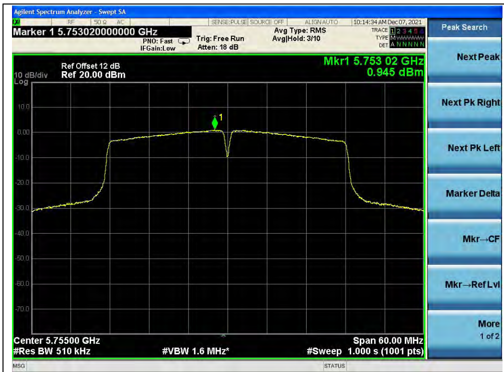
(Channel 151, 5755MHz, 802.11ac (VHT40))
