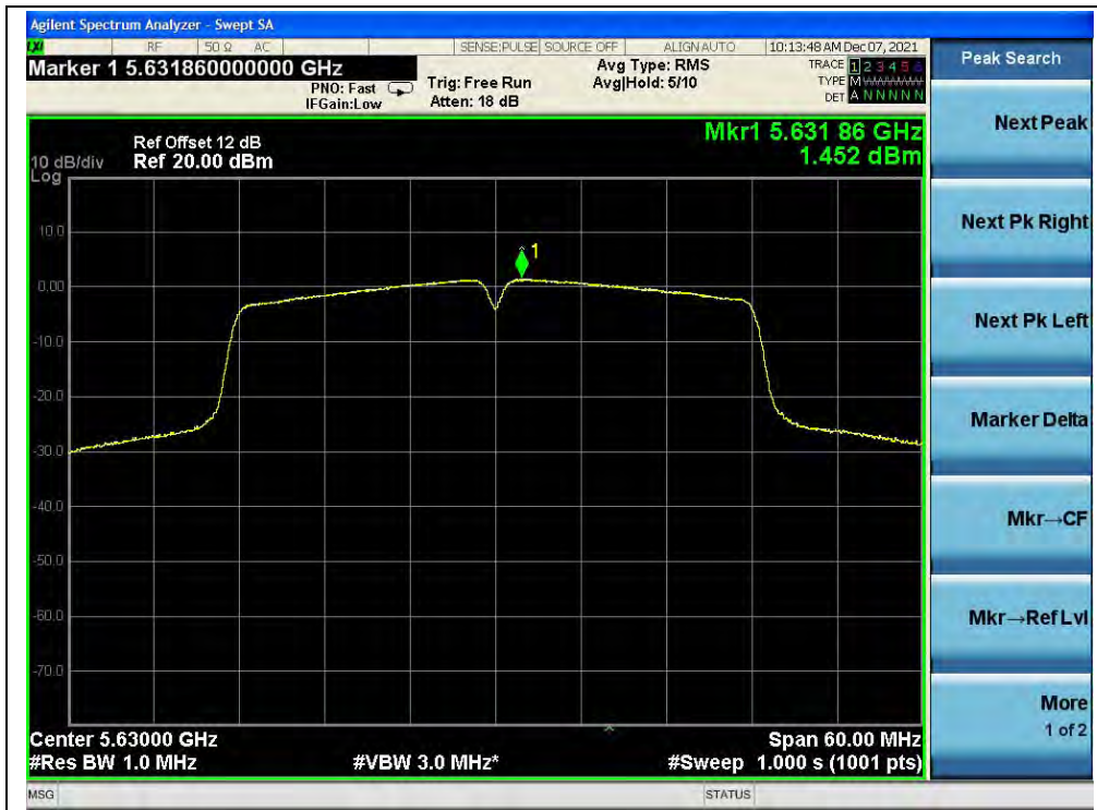
(Channel 126, 5630MHz, 802.11ac (VHT40))
