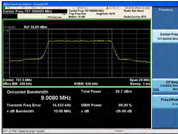
Band12 / 10MHz / High CH / QPSK
