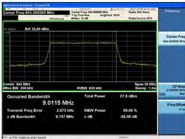
Band5 / 10MHz / High CH / QPSK
