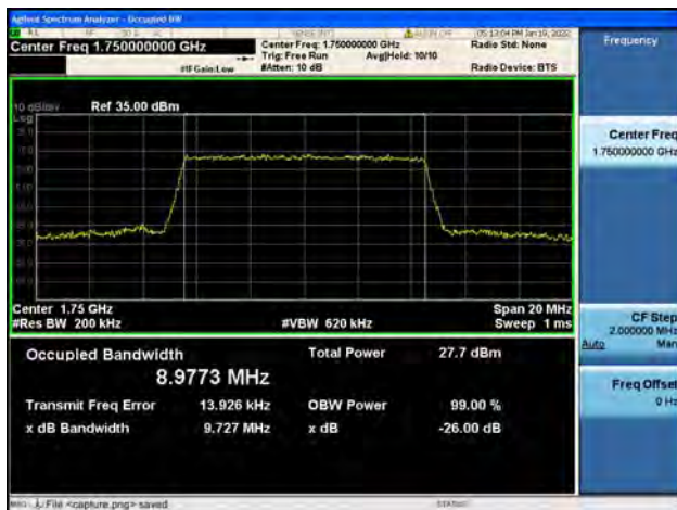
Band4 / 10MHz / High CH / QPSK
