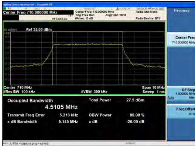
Band17 / 5MHz / High CH / QPSK
