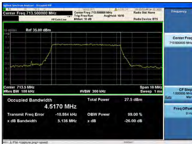
Band17 / 5MHz / High CH / QPSK
