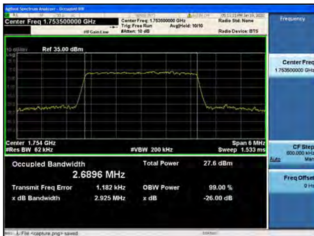
Band4 / 3MHz / High CH / QPSK
