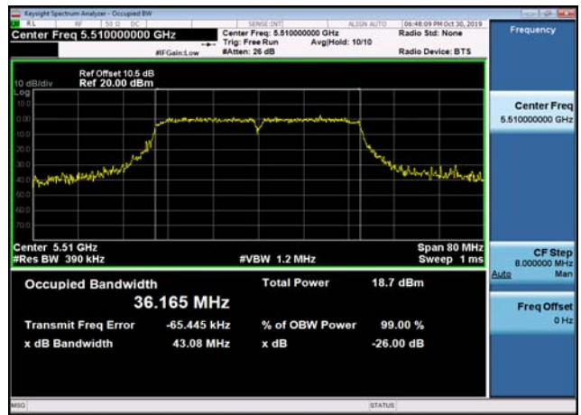
U-NII-2c 26dB Bandwidth-802.11n(40MHz),5670MHz,Ant1
