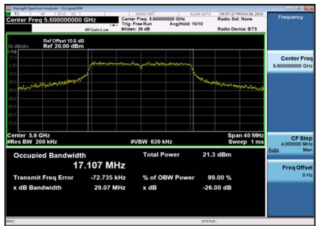
U-NII-2c 26dB Bandwidth-802.11a(20MHz),5600MHz,Ant1
