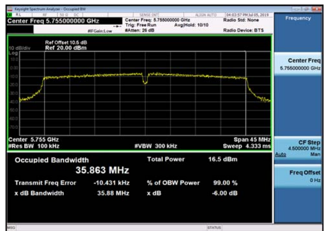
U-NII-3 6dB Bandwidth-802.11ac(80MHz) ,5775MHz,Ant1
