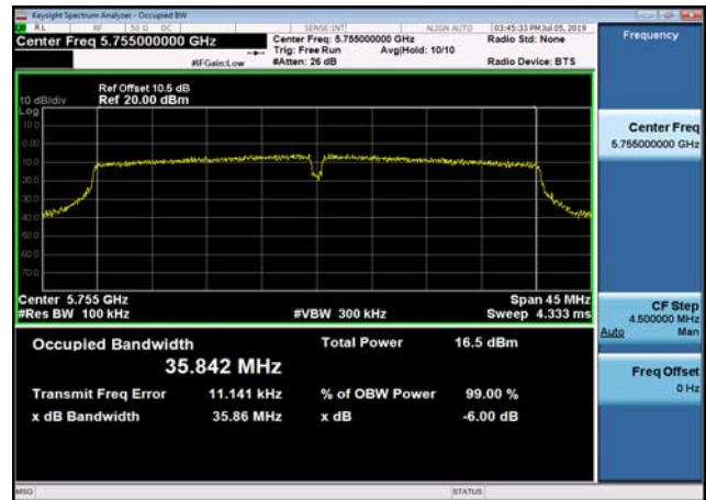
U-NII-3 6dB Bandwidth-802.11a(20MHz) ,5745MHz,Ant1
