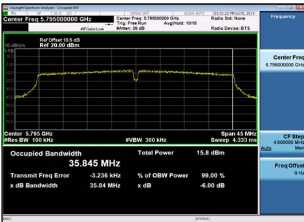
U-NII-3 6dB Bandwidth-802.11a(20MHz) ,5785MHz,Ant1
