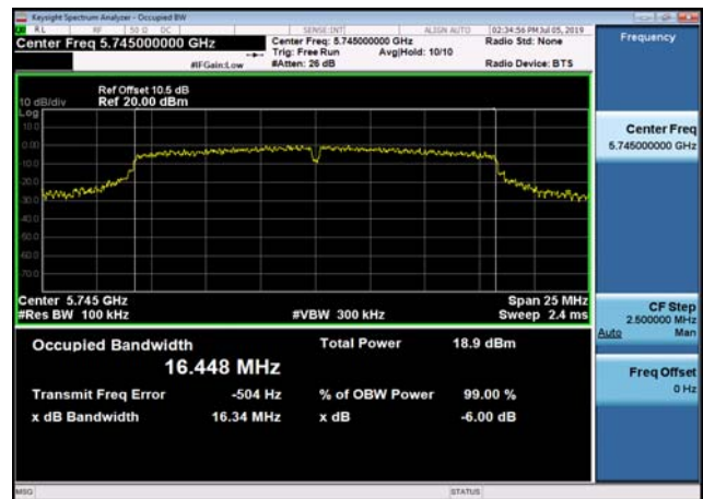
U-NII-3 6dB Bandwidth-802.11a(20MHz) ,5825MHz,Ant1
