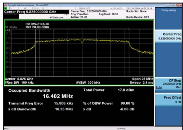
U-NII-3 6dB Bandwidth-802.11a(20MHz) ,5825MHz,Ant1
