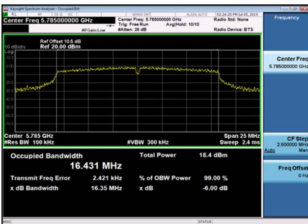
U-NII-3 6dB Bandwidth-802.11a(20MHz) ,5785MHz,Ant1
