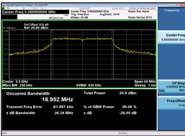
U-NII-2c 26dB Bandwidth-802.11a(20MHz),5500MHz,Ant1
