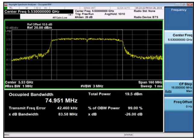
U-NII-2c 26dB Bandwidth-802.11ac(80MH z),5530MHz,Ant1
