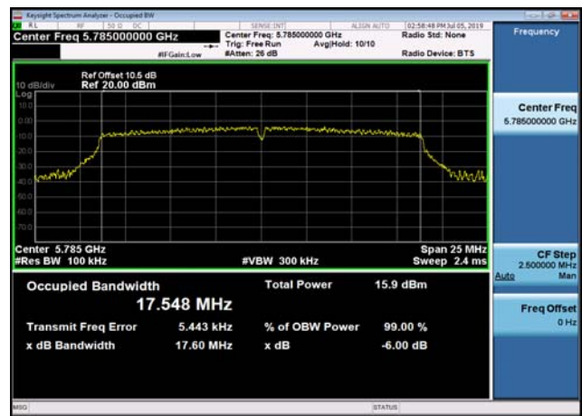
U-NII-3 6dB Bandwidth-802.11n(20MHz) ,5785MHz,Ant1
