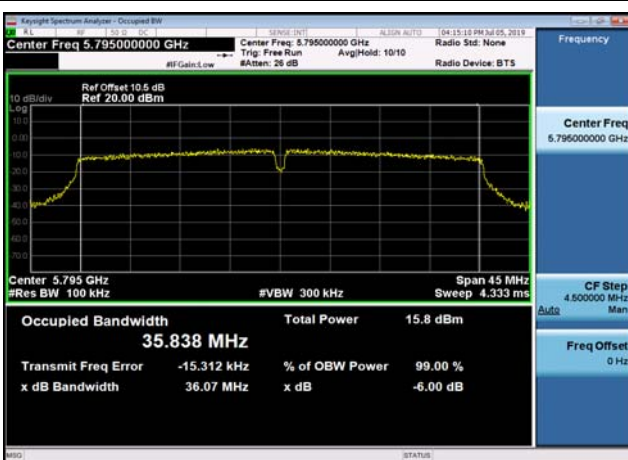
U-NII-3 6dB Bandwidth-802.11ac(40MHz) ,5795MHz,Ant1
