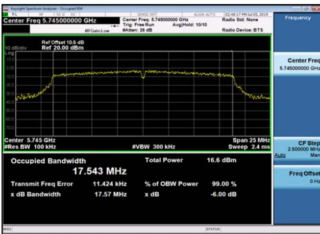
U-NII-3 6dB Bandwidth-802.11n(20MHz) ,5745MHz,Ant1
