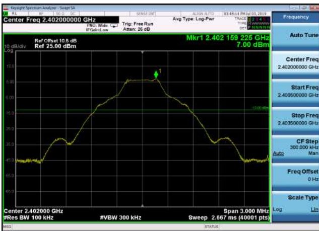
Conducted Emission: GFSK,2402,DH5 ,Reference Level
