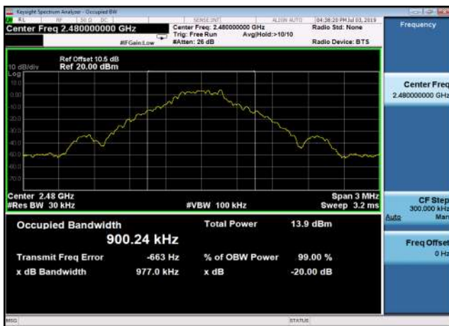
20dB Bandwidth: DQPSK,2441MHz,2DH5
