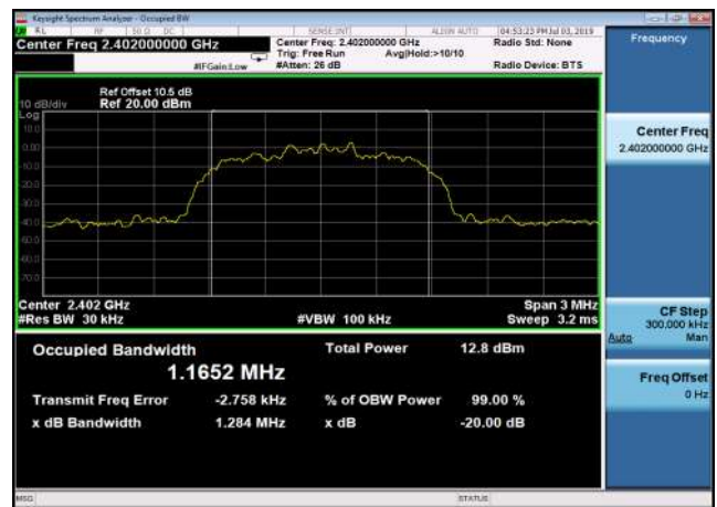
20dB Bandwidth: DQPSK,2480MHz,2DH5
