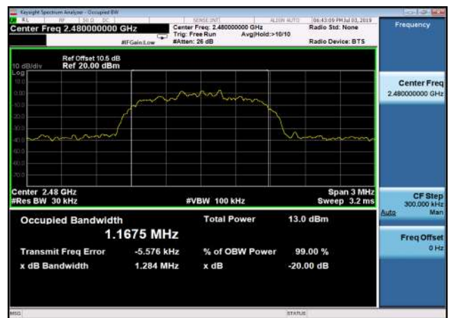
20dB Bandwidth: DQPSK,2480MHz,2DH5
