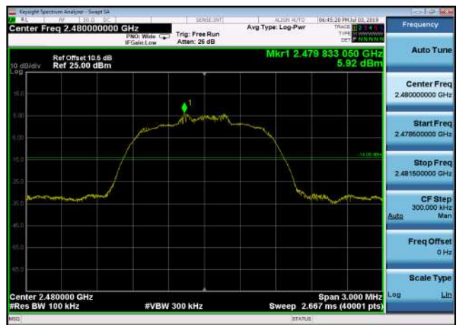
Conducted Emission: DQPSK,2480,2DH5 ,Reference Level
