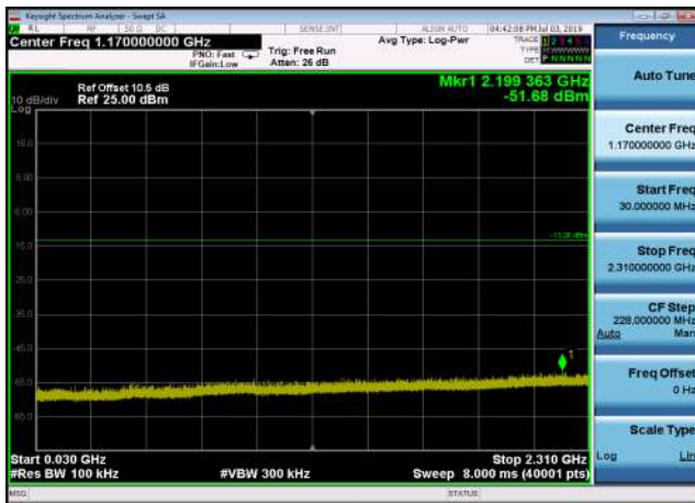
Conducted Emission: GFSK,2480,DH5 ,Reference Level
