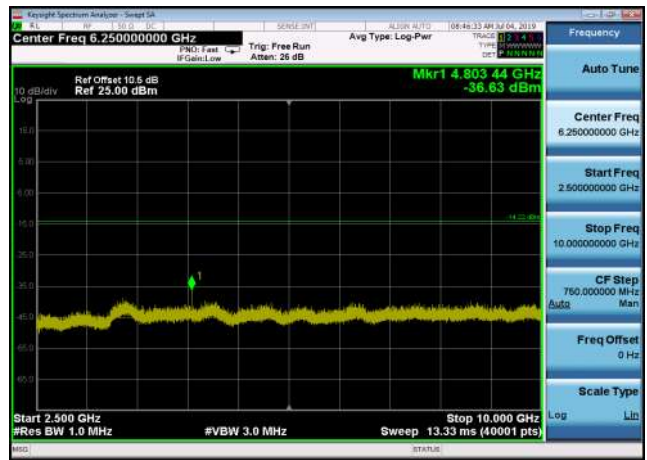
Conducted Emission: 8DPSK,2402,3DH5 ,Band Edge HoppingOFF
