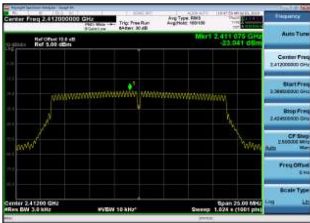
Power spectral density-802.11n(HT20) ,2462MHz
