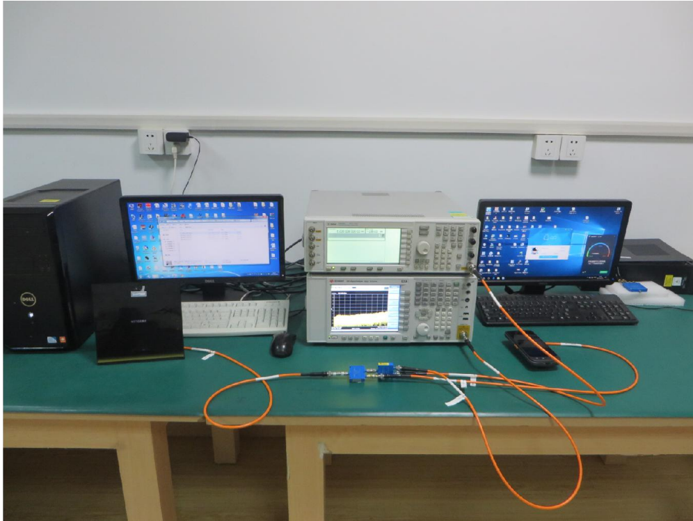
Description: DFS Test Setup
