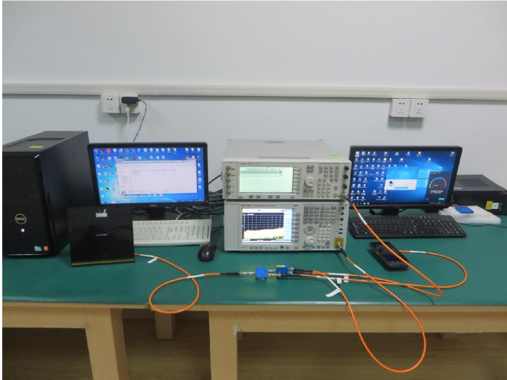
Description: DFS Test Setup
