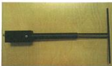
Figure 1 – MVG COMOSAR Validation Dipole
