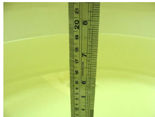
Fig 7.2 Photo of Liquid Height for Body SAR
