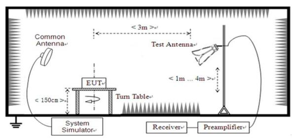
(For the test frequency above 1GHz)
