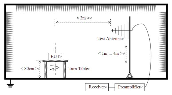
(For the test frequency from 30MHz to1GHz)
