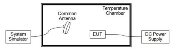
The EUT, which is powered by the DC Power Supply directly, is located in the Temperature Chamber. The EUT is commanded by the System Simulator (SS) to operate at the maximum output power i.e. Power Control Level (PCL) = 5 and Power Class = 4. A call is established between the EUT and the SS via a Common Antenna.
