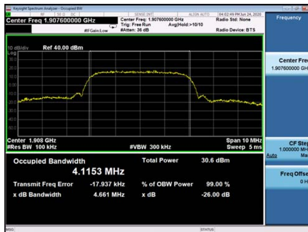
(Plot F3: WCDMA 1900MHz Channel = 9538 Occupied bandwidth)
