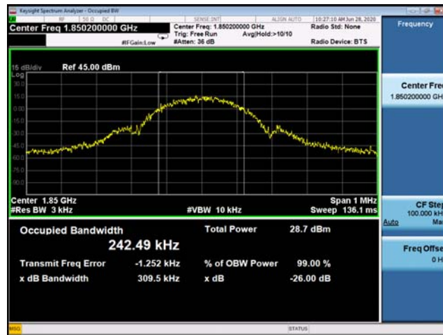
(Plot D1: EDGE 1900MHz Channel = 512 Occupied bandwidth)
