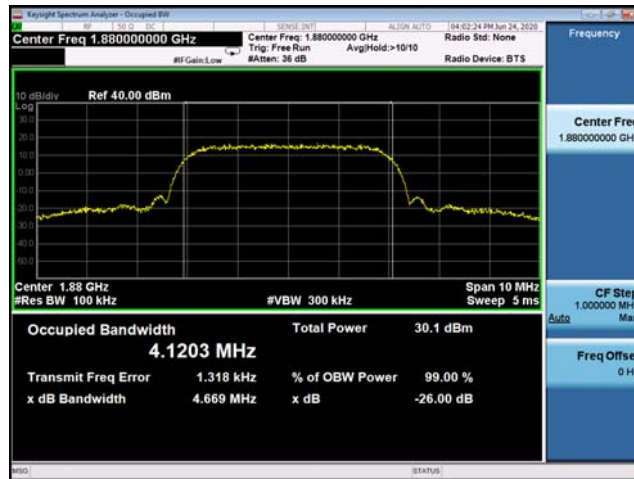
(Plot F2: WCDMA 1900MHz Channel = 9400 Occupied bandwidth)
