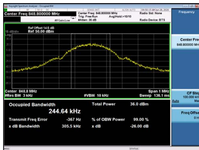
(Plot A3: GSM 850MHz Channel = 251 Occupied bandwidth)
