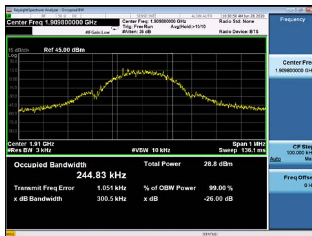
(Plot D3: EDGE 1900MHz Channel = 810 Occupied bandwidth)
