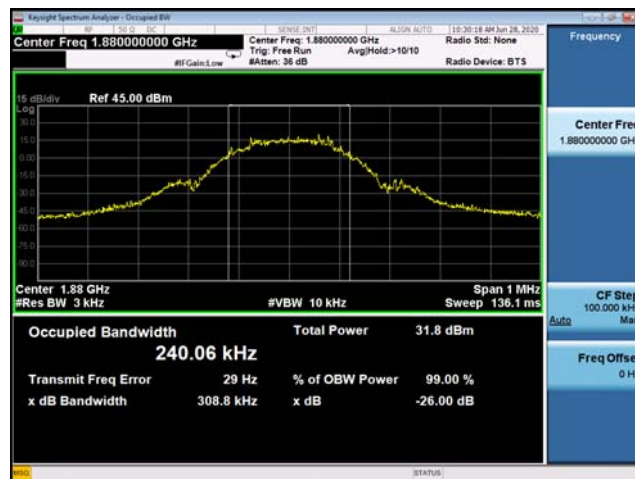
(Plot D2: EDGE 1900MHz Channel = 661 Occupied bandwidth)
