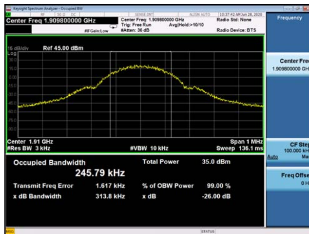
(Plot B3: GSM 1900MHz Channel = 810 Occupied bandwidth)
