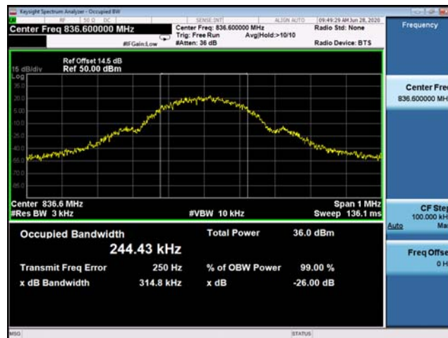
(Plot A2: GSM 850MHz Channel = 190 Occupied bandwidth)
