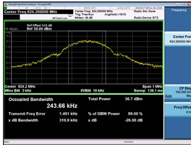
(Plot A1: GSM 850MHz Channel = 128 Occupied bandwidth)
