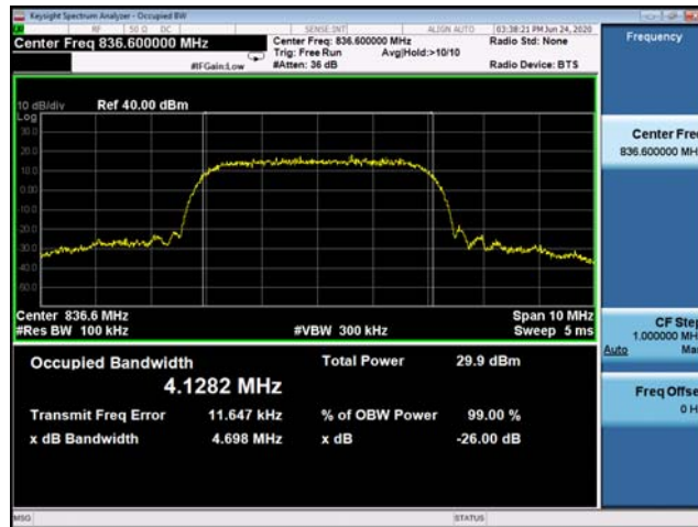
(Plot E2: WCDMA 850MHz Channel = 4183 Occupied bandwidth)
