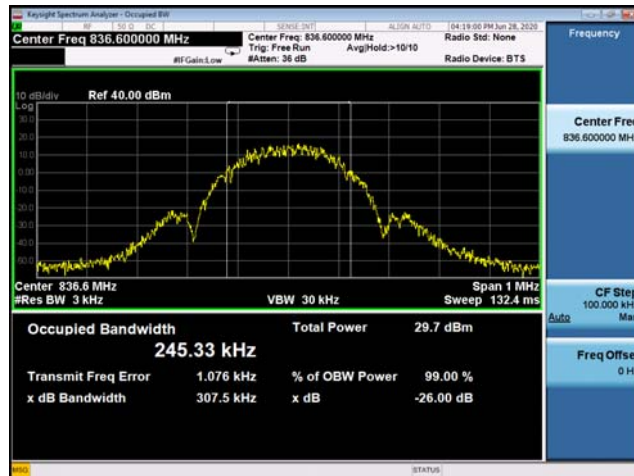
(Plot C2: EDGE 850MHz Channel = 190 Occupied bandwidth)
