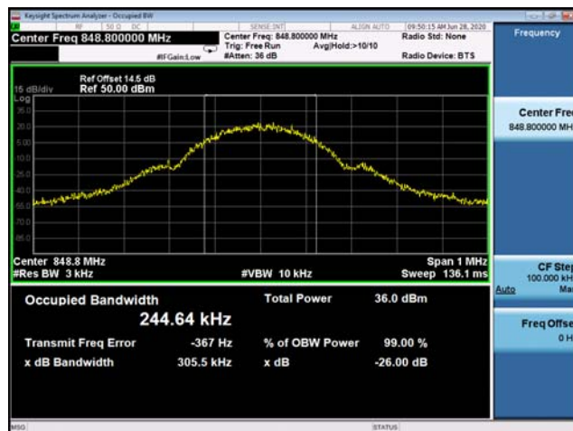
(Plot C3: EDGE 850MHz Channel = 251 Occupied bandwidth)
