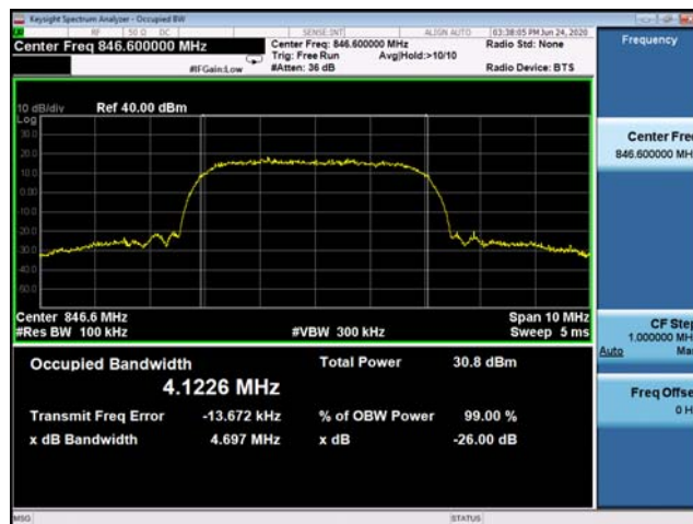
(Plot E3: WCDMA 850MHz Channel = 4233 Occupied bandwidth)
