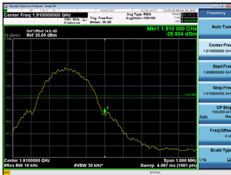
(Plot D: GSM 1900 Channel = 810)
