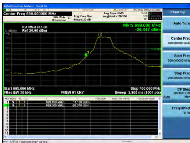
Band12 / 3MHz / Low CH / QPSK / 1 RB
