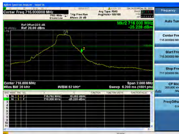
Band12 / 3MHz / Low CH / QPSK / 1 RB
