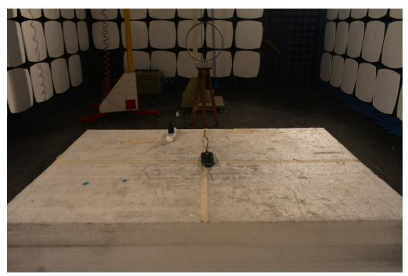
3. Radiated emission (9KHz-30MHz)
