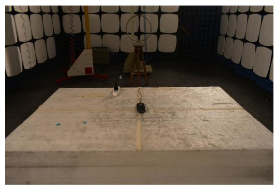
3. Radiated emission (9KHz-30MHz)
