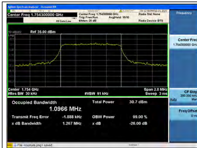
Band4 / 1.4MHz / QPSK/ High CH
