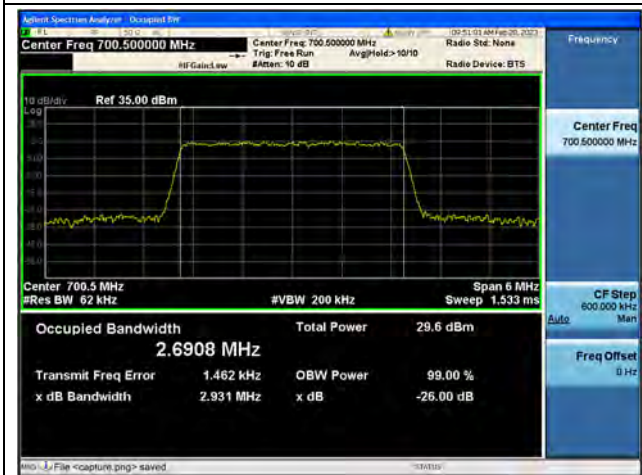
Band12 / 3MHz / 16QAM/ Low CH
