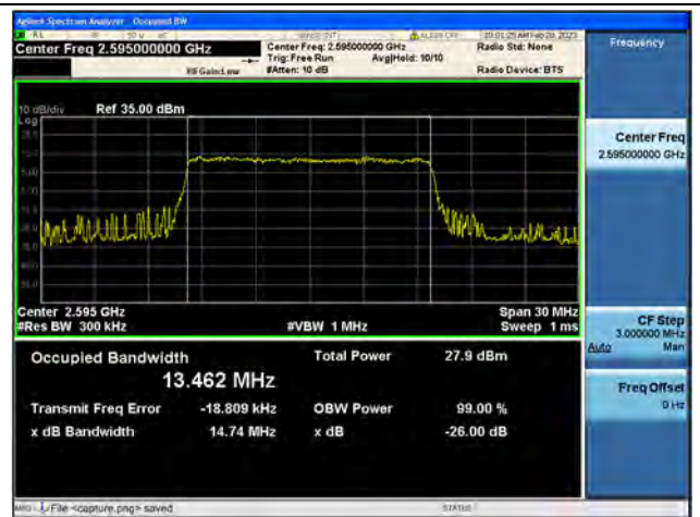
Band38 / 15MHz / 64QAM/ Mid CH
