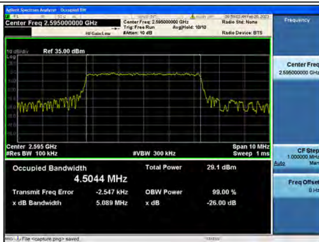
Band38 / 5MHz / 16QAM/ Mid CH
