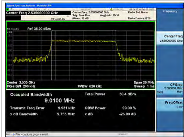
Band7 / 10MHz / QPSK/ Mid CH
