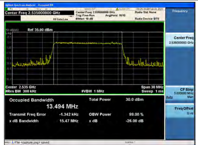
Band7 / 15MHz / QPSK/ Mid CH
