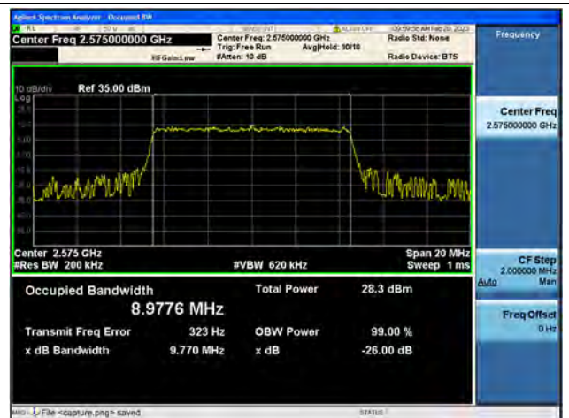
Band38 / 10MHz / 64QAM/ Low CH
