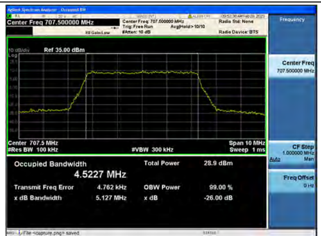
Band12 / 5MHz / 64QAM/ Mid CH
