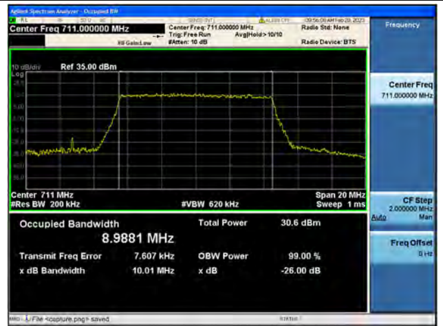
Band17 / 10MHz / QPSK/ High CH
