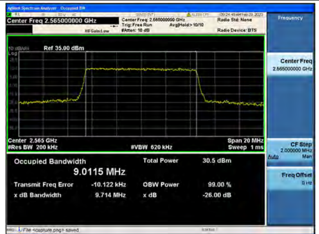
Band7 / 10MHz / QPSK/ High CH
