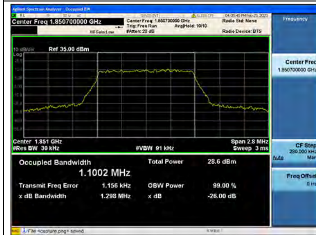
Band2 / 1.4MHz / 64QAM/ Low CH
