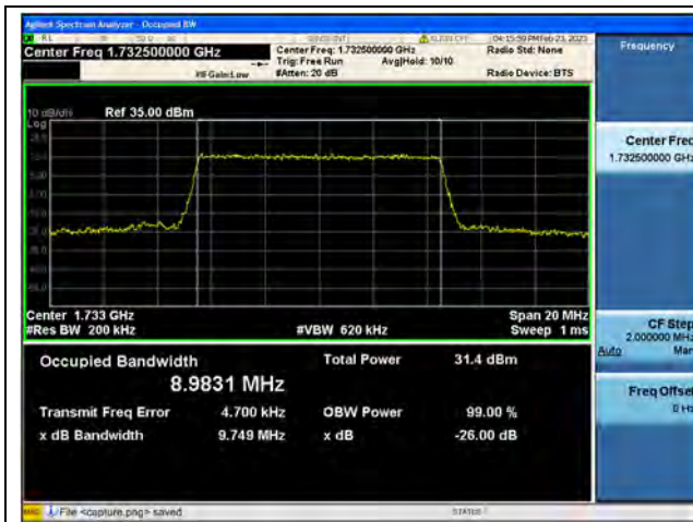
Band4 / 10MHz / QPSK/ Mid CH
