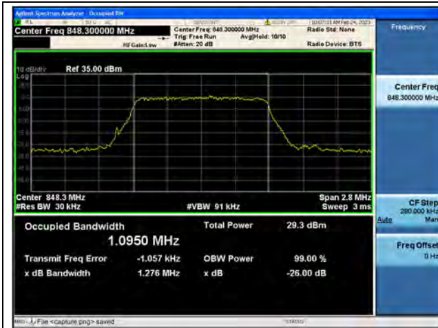
Band5 / 1.4MHz / QPSK/ High CH
