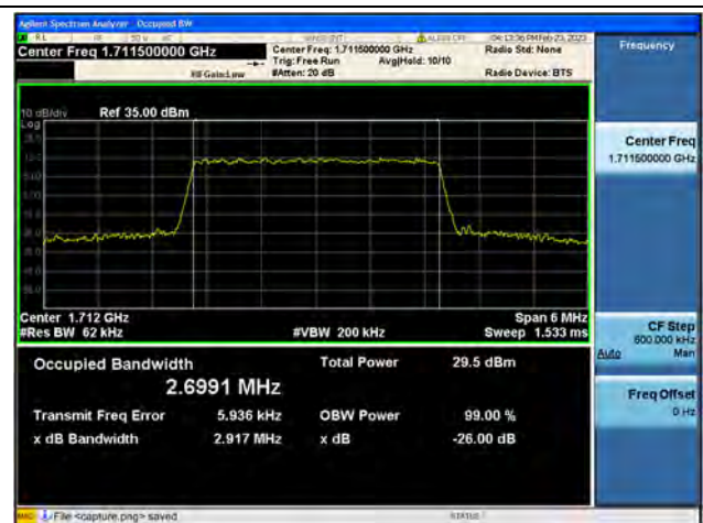
Band4 / 3MHz / 64QAM/ Low CH
