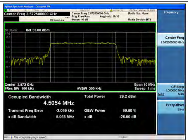
Band38 / 5MHz / 16QAM/ Low CH
