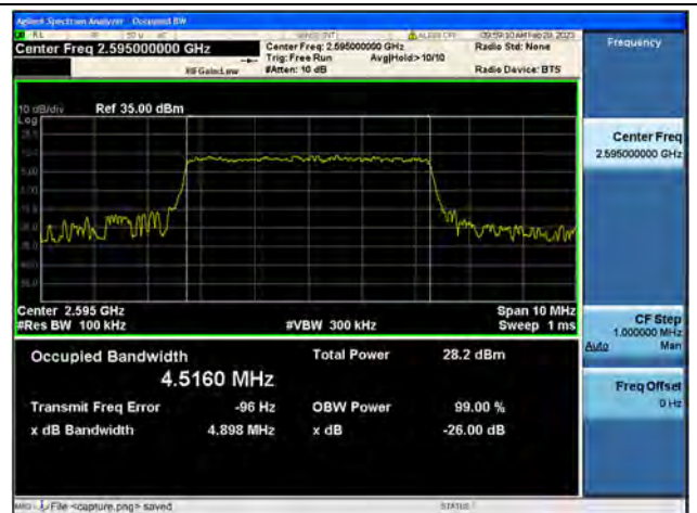
Band38 / 5MHz / 64QAM/ Mid CH
