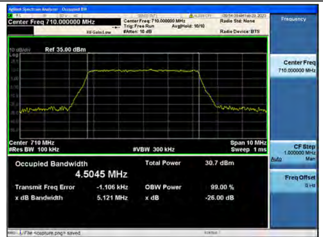
Band17 / 5MHz / QPSK/ Mid CH
