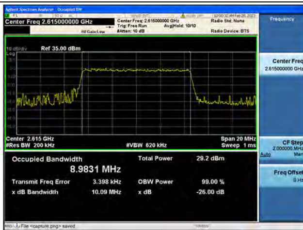
Band38 / 10MHz / 16QAM / High CH
