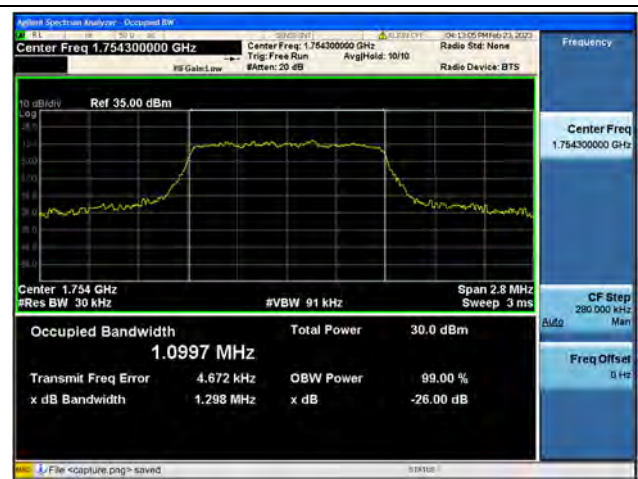
Band4 / 1.4MHz / 16QAM/ High CH
