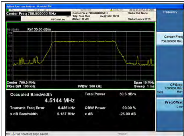
Band17 / 5MHz / QPSK/ Low CH
