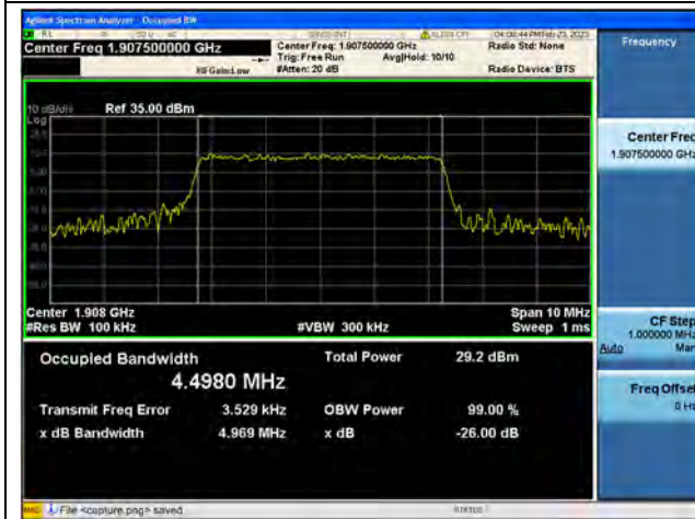
Band2 / 5MHz / 64QAM/ High CH
