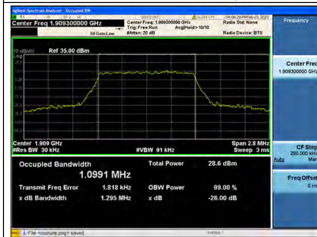
Band2 / 1.4MHz / 64QAM/ High CH
