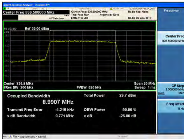
Band5 / 10MHz / 64QAM/ Mid CH
