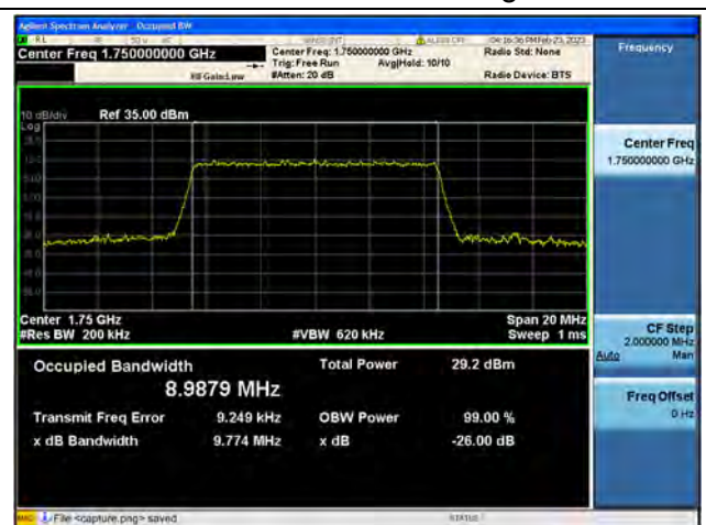
Band4 / 10MHz / 64QAM/ High CH
