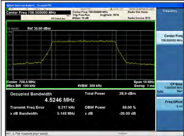
Band17 / 5MHz / 64QAM/ Low CH
