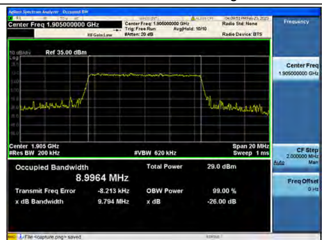
Band2 / 10MHz / 64QAM/ High CH
