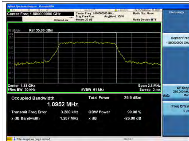
Band2 / 1.4MHz / 16QAM/ Mid CH
