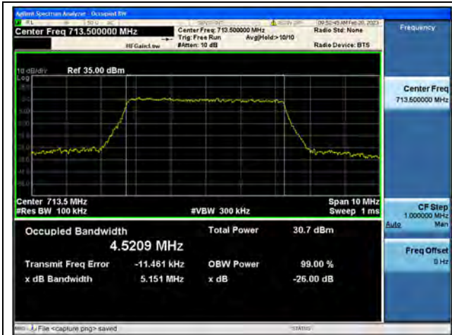
Band12 / 5MHz / QPSK/ High CH
