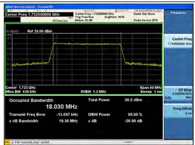
Band4 / 20MHz / 16QAM/ Mid CH
