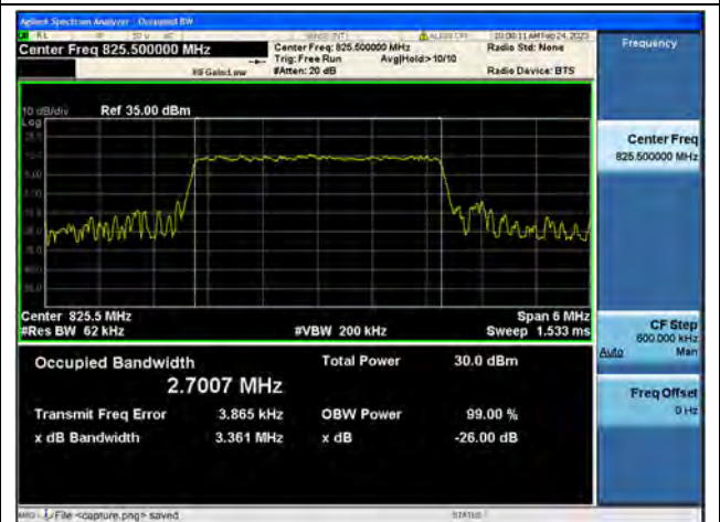
Band5 / 3MHz / 64QAM/ Low CH
