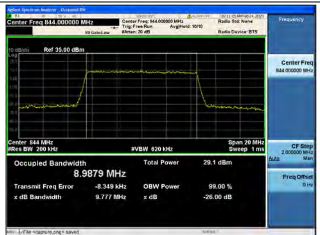
Band5 / 10MHz / 64QAM/ High CH
