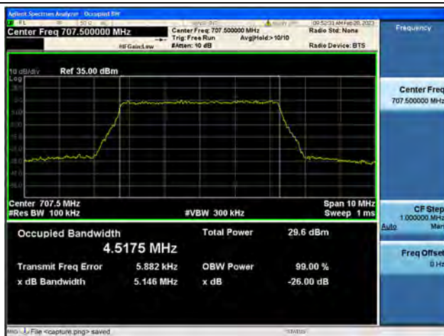
Band12 / 5MHz / 16QAM/ Mid CH
