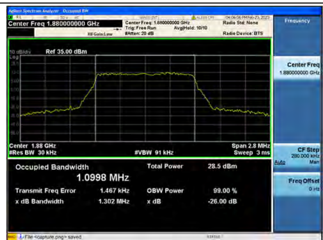
Band2 / 1.4MHz / 64QAM/ Mid CH
