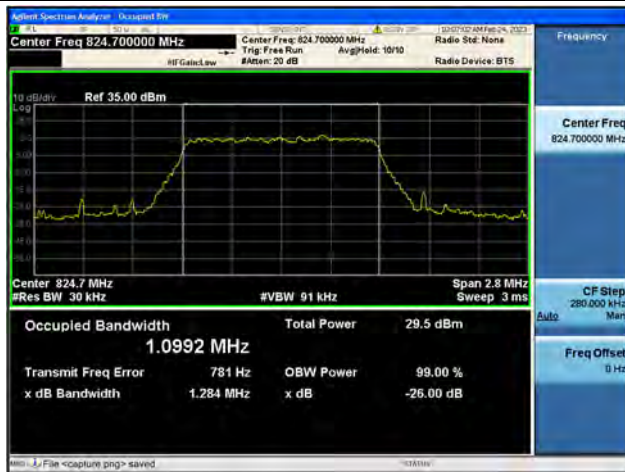
Band5 / 1.4MHz / 64QAM/ Low CH
