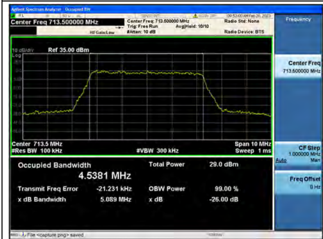
Band12 / 5MHz / 64QAM/ High CH
