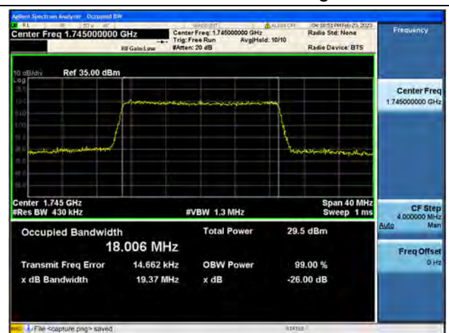
Band4 / 20MHz / 64QAM/ High CH
