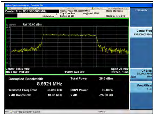
Band5 / 10MHz / QPSK/ Mid CH
