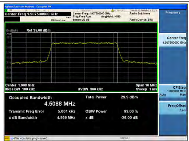
Band2 / 5MHz / 16QAM/ High CH
