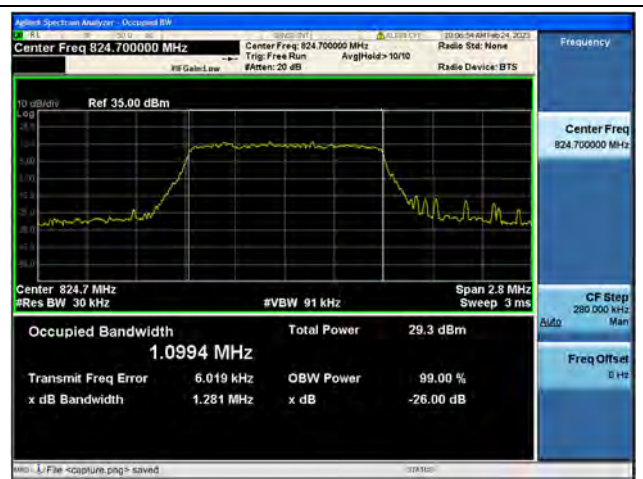
Band5 / 1.4MHz / 16QAM/ Low CH
