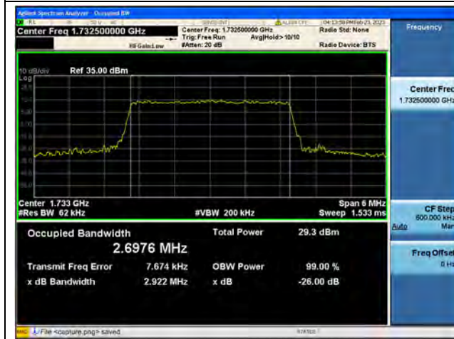
Band4 / 3MHz / 64QAM/ Mid CH
