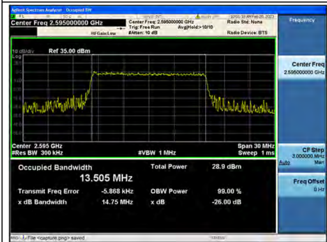
Band38 / 15MHz / 16QAM/ Mid CH
