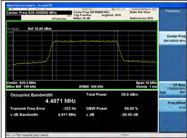
Band5 / 5MHz / 64QAM/ Low CH
