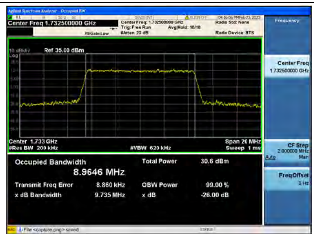
Band4 / 10MHz / 16QAM/ Mid CH
