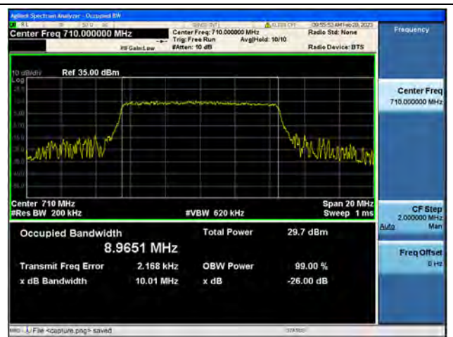
Band17 / 10MHz / 16QAM/ Mid CH
