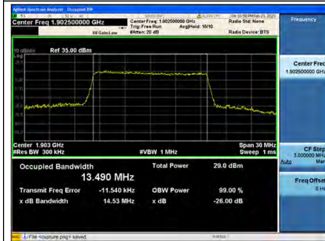
Band2 / 15MHz / 64QAM/ High CH
