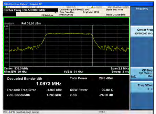
Band5 / 1.4MHz / QPSK/ Mid CH
