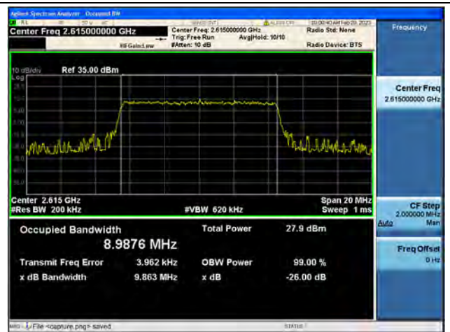
Band38 / 10MHz / 64QAM / High CH
