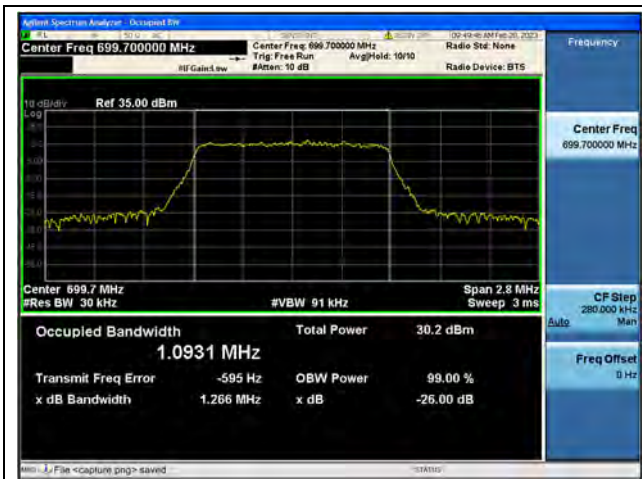
Band12 / 1.4MHz / QPSK/ Low CH
