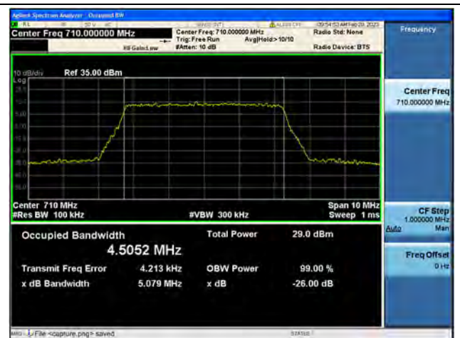
Band17 / 5MHz / 64QAM/ Mid CH
