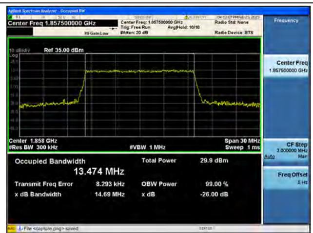
Band2 / 15MHz / 16QAM/ Low CH
