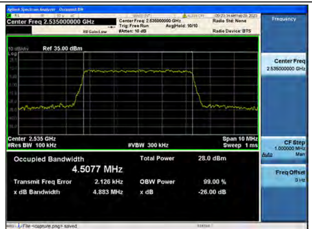
Band7 / 5MHz / 64QAM/ Mid CH
