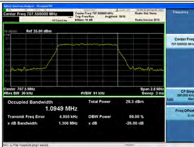
Band12 / 1.4MHz / 16QAM/ Mid CH
