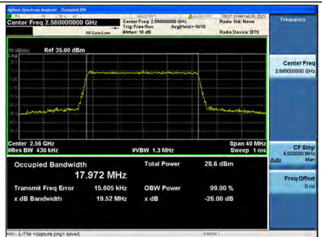
Band7 / 20MHz / 64QAM/ High CH
