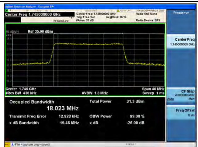
Band4 / 20MHz / QPSK/ High CH
