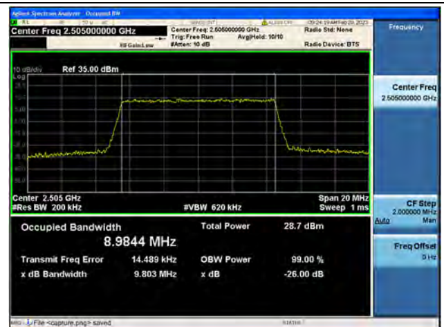
Band 7 / 10MHz / 64QAM / Low CH
