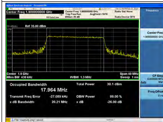
Band2 / 20MHz / 16QAM/ High CH
