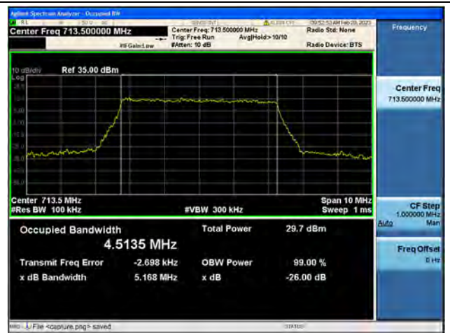
Band12 / 5MHz / 16QAM/ High CH
