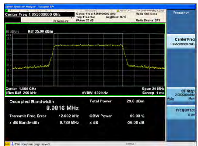
Band2 / 10MHz / 64QAM/ Low CH
