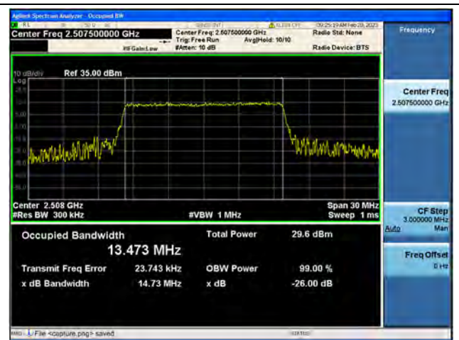
Band7 / 15MHz / 16QAM/ Low CH
