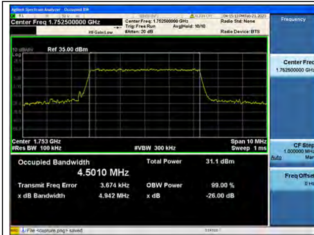
Band4 / 5MHz / QPSK/ High CH
