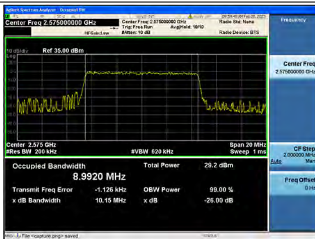
Band38 / 10MHz / 16QAM/ Low CH
