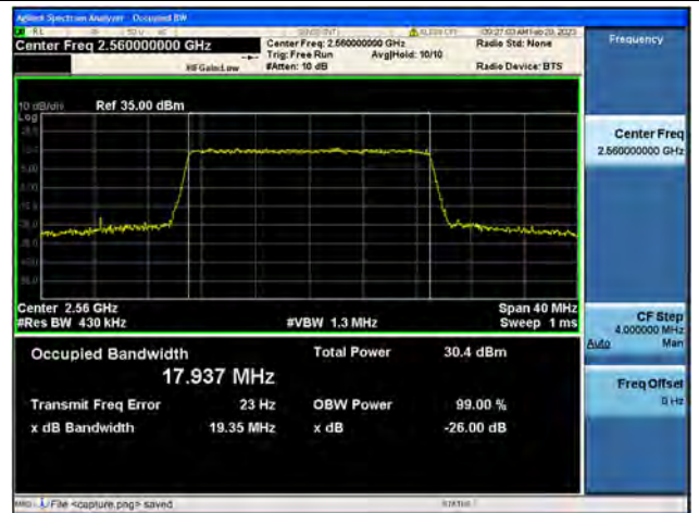
Band7 / 20MHz / QPSK/ High CH
