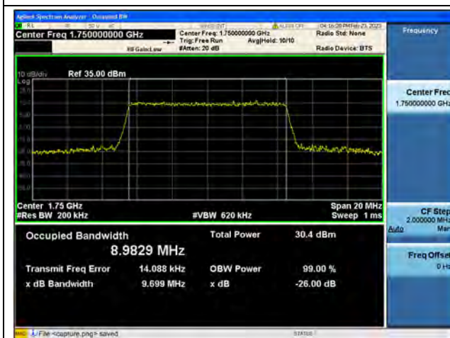
Band4 / 10MHz / 16QAM/ High CH
