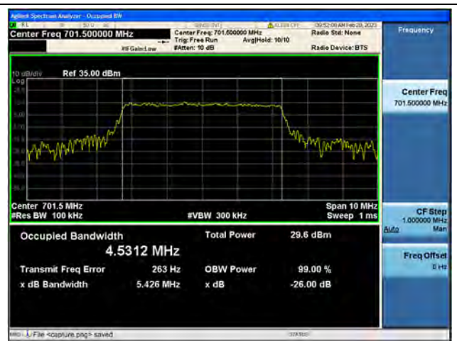
Band12 / 5MHz / 16QAM/ Low CH
