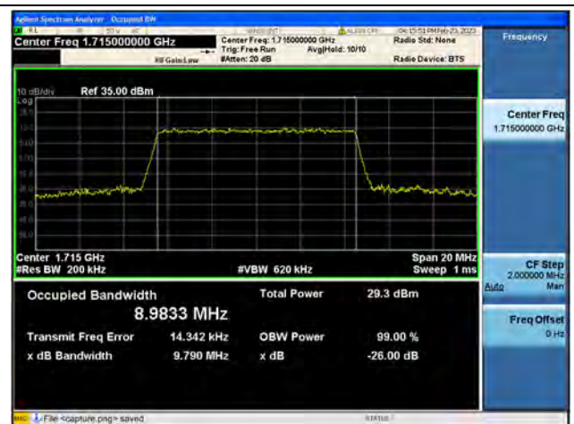
Band4 / 10MHz / 64QAM/ Low CH
