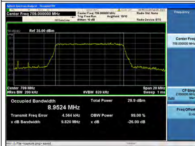
Band17 / 10MHz / 16QAM/ Low CH
