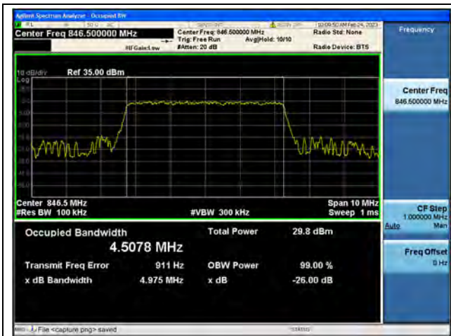
Band5 / 5MHz / QPSK/ High CH
