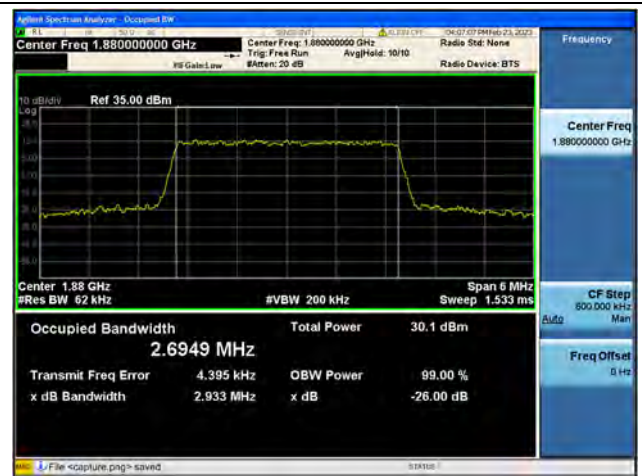
Band2 / 3MHz / 16QAM/ Mid CH
