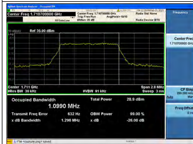
Band4 / 1.4MHz / 64QAM/ Low CH
