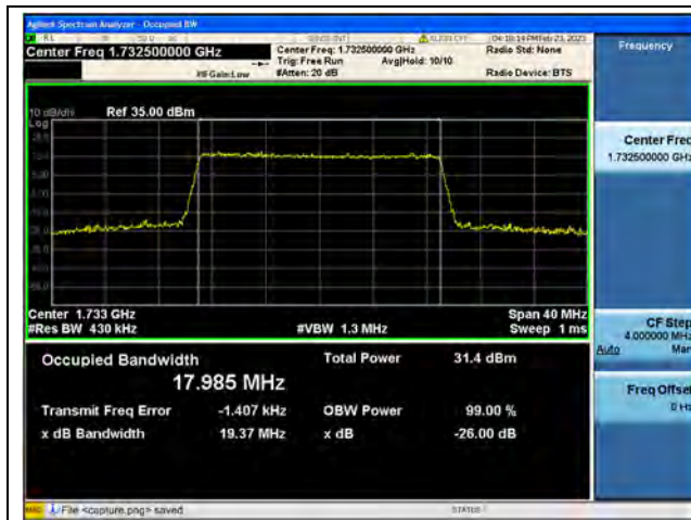
Band4 / 20MHz / QPSK/ Mid CH
