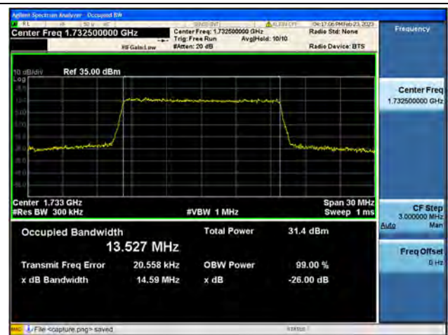
Band4 / 15MHz / QPSK/ Mid CH
