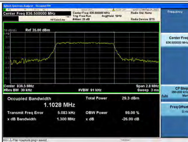
Band5 / 1.4MHz / 16QAM/ Mid CH
