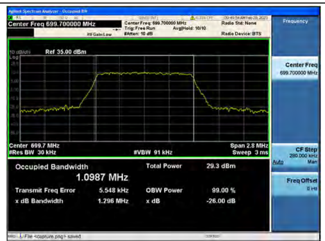
Band12 / 1.4MHz / 16QAM/ Low CH
