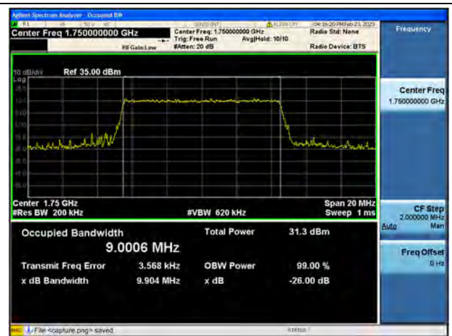
Band4 / 10MHz / QPSK/ High CH
