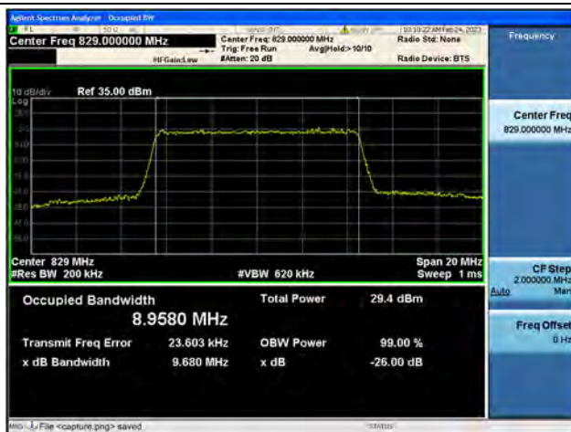
Band5 / 10MHz / 16QAM/ Low CH
