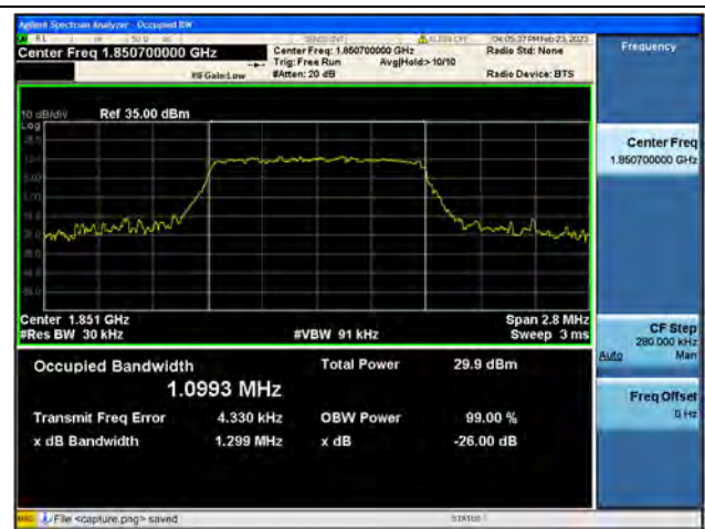
Band2 / 1.4MHz / 16QAM/ Low CH
