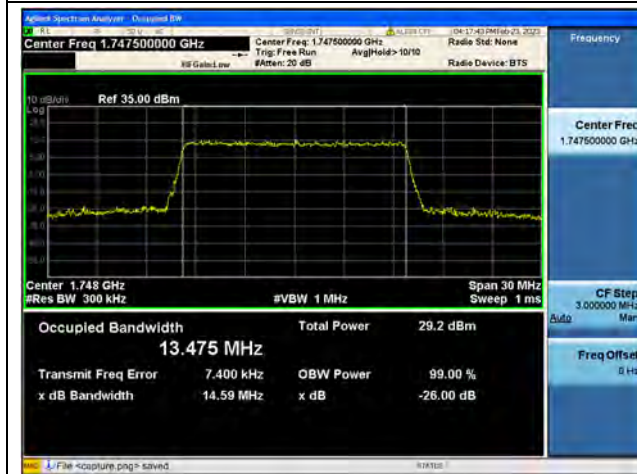
Band4 / 15MHz / 64QAM/ High CH
