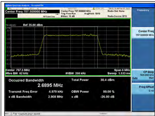
Band12 / 3MHz / QPSK/ Mid CH
