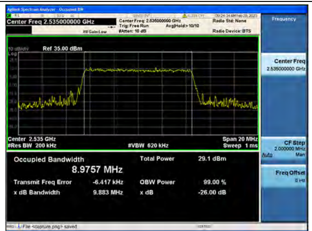
Band7 / 10MHz / 16QAM/ Mid CH
