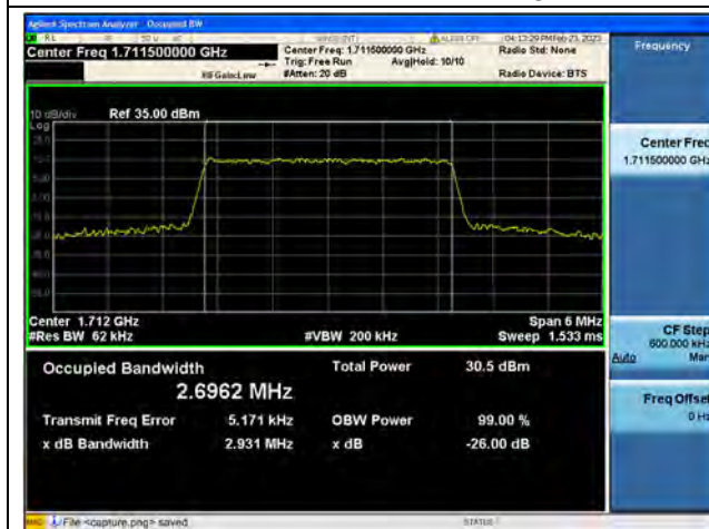
Band4 / 3MHz / 16QAM/ Low CH
