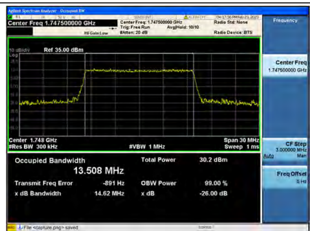
Band4 / 15MHz / 16QAM/ High CH
