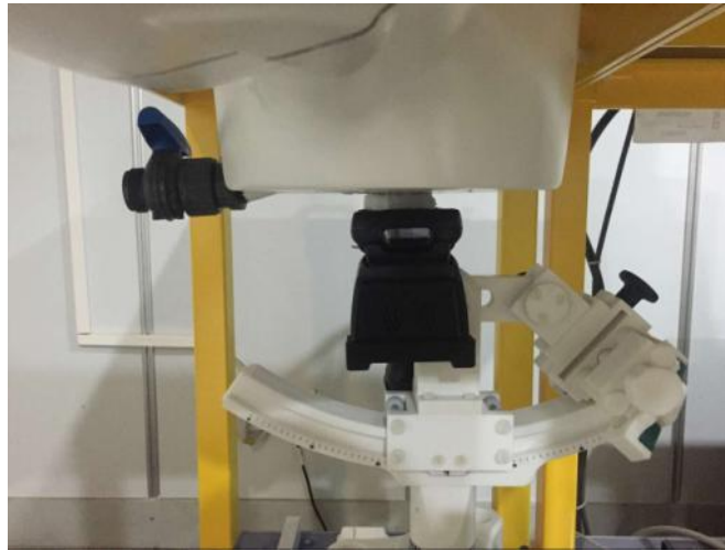
Fig.13 RFID Body (Face upside,10mm separation)
