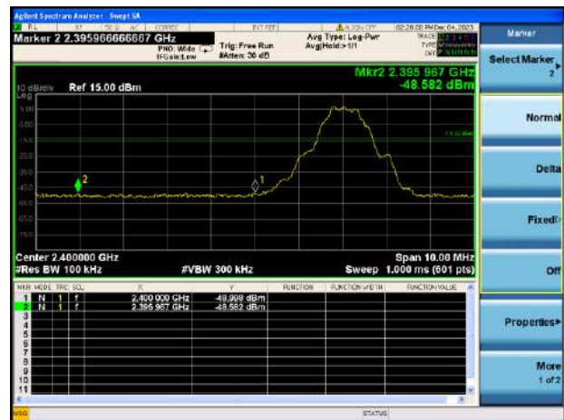
GFSK (BLE 1Mbps) HIGH CHANNEL, BAND EDGE
