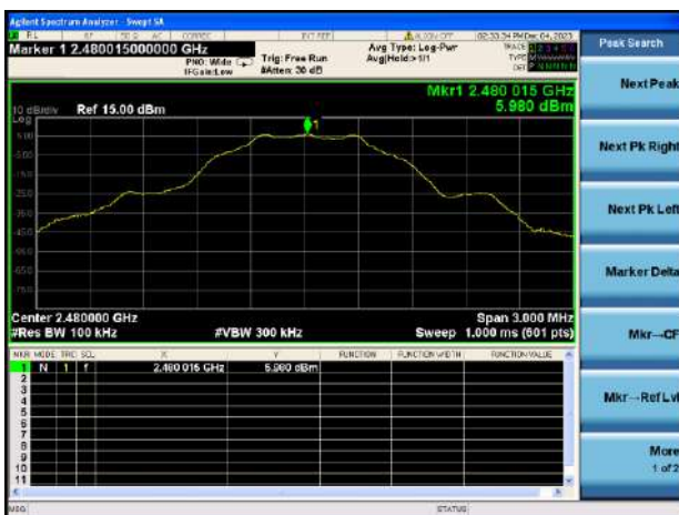
GFSK (BLE 1Mbps) HIGH CHANNEL, CARRIER LEVEL
