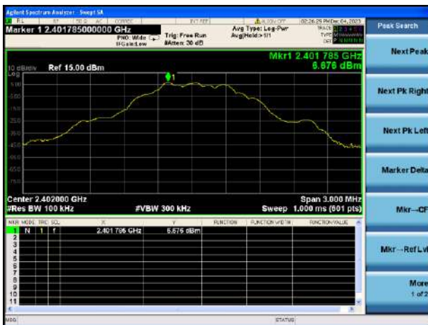
GFSK (BLE 1Mbps) LOW CHANNEL, CARRIER LEVEL
