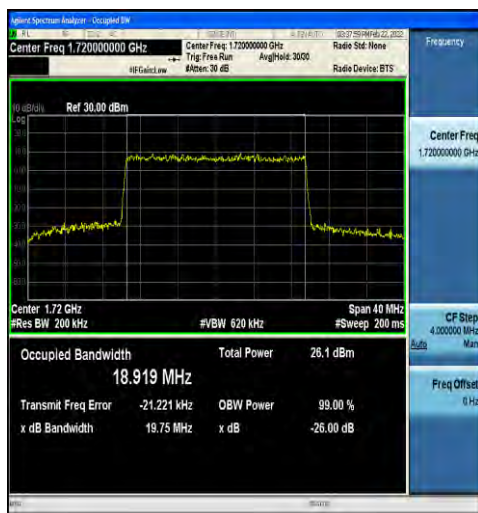
1-N66-15-20-L-9-CP-256QAM-Outer_Full-106@0-An t1-18.919-19.75-≤20-PASS
