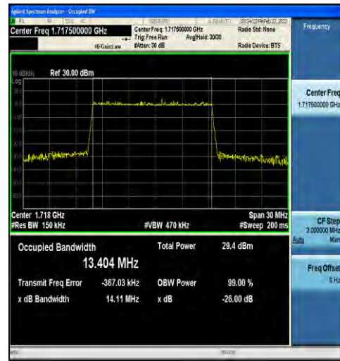
1-N66-15-15-L-4-DFT-64QAM-Outer_Full-75@0-Ant 1-13.404-14.11-≤15-PASS
