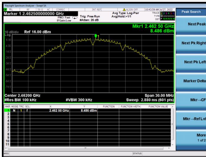
802.11b CHANNEL 11, CARRIER LEVEL
