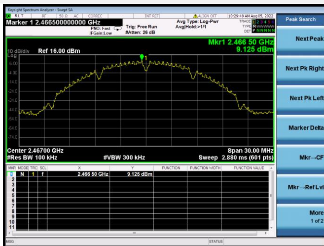
802.11b CHANNEL 12, CARRIER LEVEL
