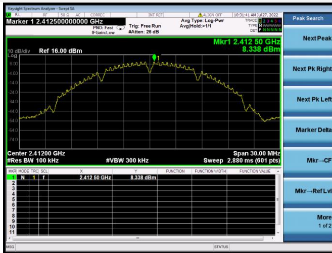
802.11b CHANNEL 1, CARRIER LEVEL
