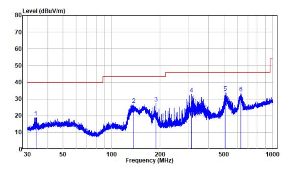
Site : chamber Condition: 3m HORIZONTAL Job No. : SZNS220303-07022E-RF Test Mode: Base Charging
