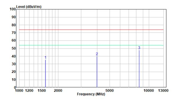
Site : chamber Condition: 3m VERTICAL Job No. : SZNS220303-07022E-RF Test Mode: Base Charging
