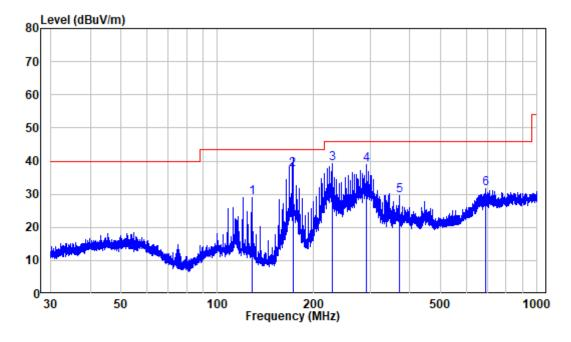
Site : chamber Condition: 3m HORIZONTAL Job No. : SZNS220303-07022E-RF Test Mode: Direct charging
