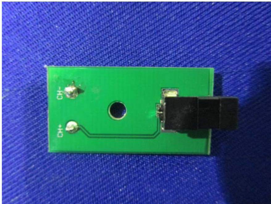
EUT –Charger Base Board Top View
