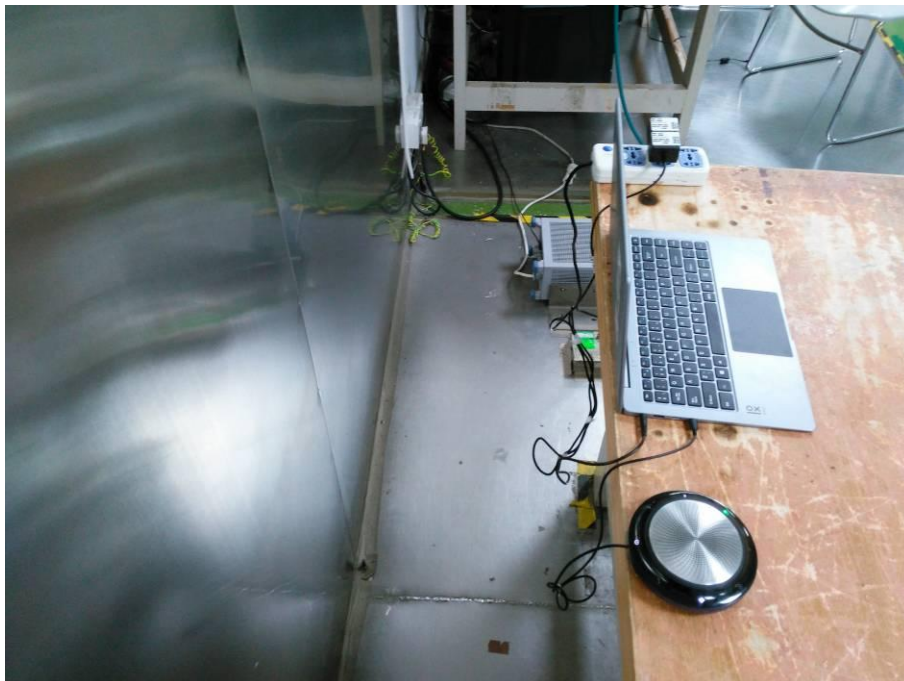
Conducted Emissions - Side View
