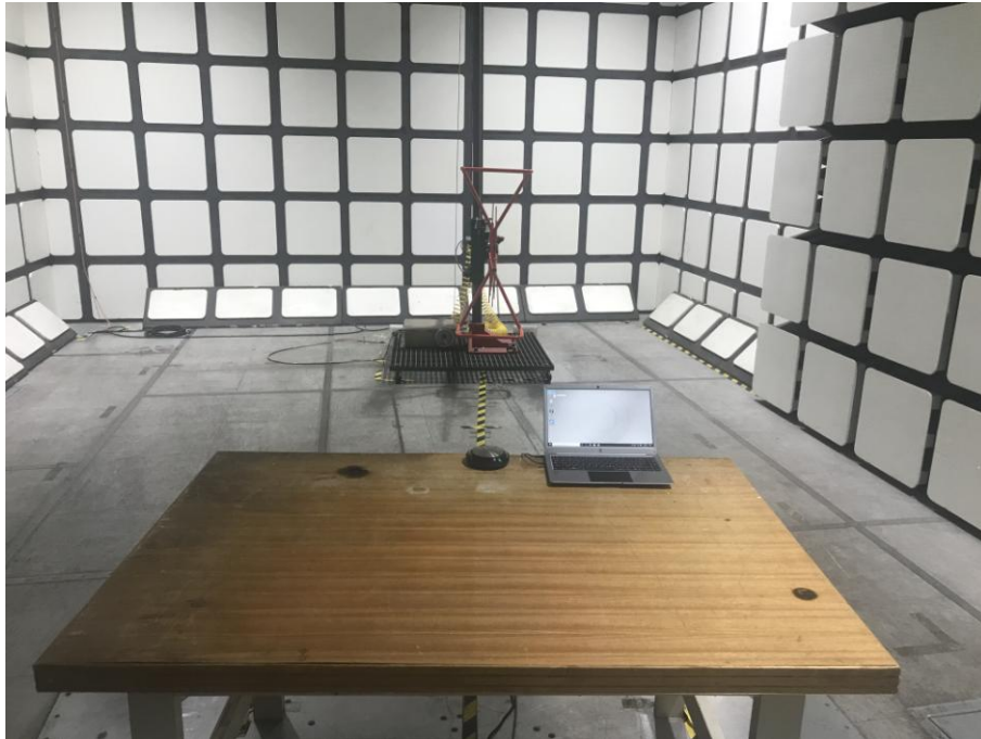
Radiated Emissions – Front View (Below 1 GHz)
